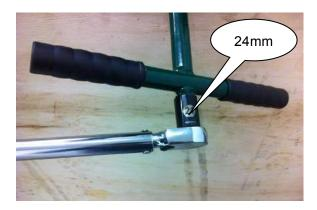
Proper blade tension is achieved when a 24mm socket is used on a torque wrench to tighten the "T" handle to 35 ft-lbs torque. See above right image.
