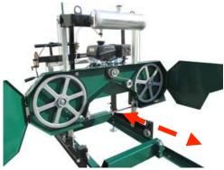
Remove the tension in the blade by turning the "T" handle in the counter-clockwise direction and then open the blade guard cover. The blade should now be loose and free to pull straight out the front.
