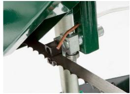
Insert the lube tank line through the hole in the bottom of the saw head as shown above. Use a 16mm socket to secure the copper end in position. Do not over tighten or crush the copper end.
