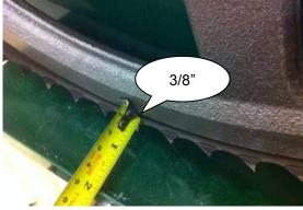
Re-tension the blade by turning the "T" handle a full turn in the clockwise direction. Wearing gloves, spin the bandwheel with your hand and observe how the blade has changed tracking. Measure the distance again and repeat the above step to further compensate if required. The ideal measurement is 3/8" or check for the back of the blade to be flush with the back of the bandwheel.
