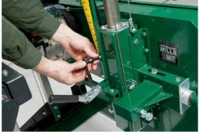
Install the square indicator rod to the sawmill using the two bolts and tighten using a 10mm socket.
