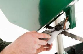
Using a piece of paper in between the blade and blade guide blocks, tighten the allen key bolts.
