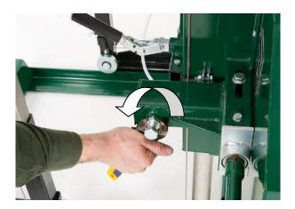
Loosen the tracking alignment locking nut with an adjustable wrench.
