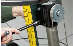
Place the measuring scale bracket as shown above and insert bolts and nuts. It is important to alternate tightening of the nuts (top then bottom) to ensure the black round clamp begins to compress evenly on both the top and bottom until flanges meet at outer edge. Tighten nuts using a 13mm socket.
