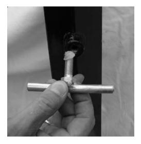
Add grease to all "T" handle threads on the sawmill.
