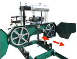
Remove the tension in the blade by turning the "T" handle in the counter-clockwise direction and then open the blade guard cover. The blade should now be loose and free to pull straight out the front. The new blade can now be installed, guards closed and proper blade tension set.
