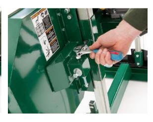
To adjust the left side of the sawmill, again start by taking the tension off of the blade by turning the "T" handle one turn in the counter-clockwise direction. Using a 17mm wrench, loosen the "vertical nut" a ½ turn. Do the same on the "bottom vertical nut". Next, loosen both "vertical bolts" a ½ turn. This will take the clamping force off of the bandwheel shaft caused by these two bolts and allow it to move freely in the following steps.
