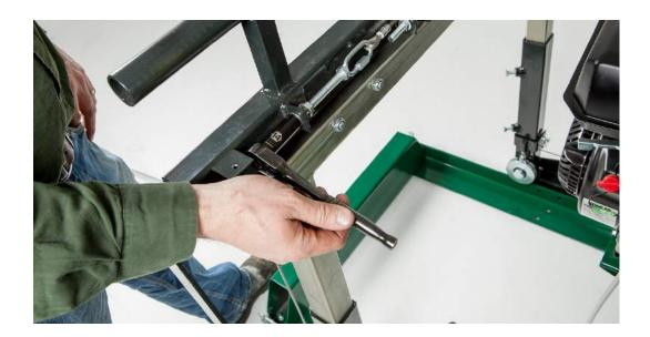
Using a 14mm socket, turn the nut either clockwise to raise one side of the saw head or counter-clockwise to lower one side of the saw head. Double check the blade height as discussed in the previous step. Once measurement is consistent on both sides, tighten the corresponding nut to clamp securely against tab.
