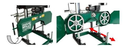
Remove the tension in the blade by turning the "T" handle in the counter-clockwise direction and then open the blade guard cover. The blade should now be loose and free to pull straight out the front. The new blade can now be installed, guards closed and proper blade tension set.
