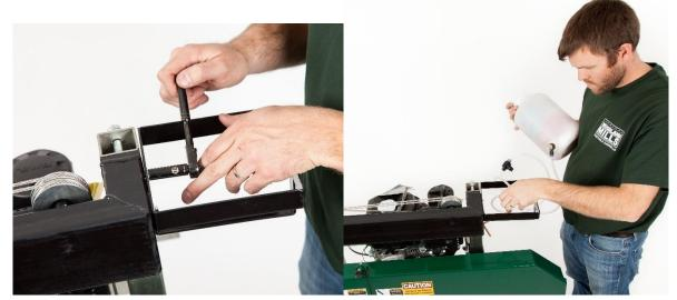
Attach lubrication tank bracket to the left side of the sawmill cross support using the two bolts provided and tighten with a 10mm socket. The lube tank and hose can also be rested into the bracket.
