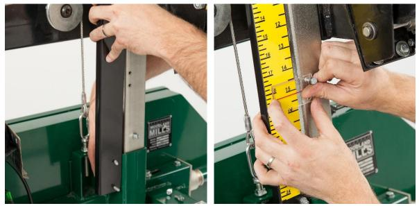
Attach the metal scale bracket to the sawmill head using the two nuts and bolts provided. Use a 10mm socket to tighten. Attach the scale indicator to the post with the two bolts provided and tighten with a 10mm socket. The magnetic log scale can also be placed on the bracket.
