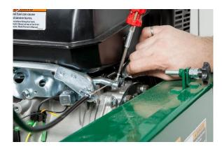
With the throttle lever in the idle position/fully open, pull the cable tight at the engine and tighten the screw to hold it in place. This will take all of the slack out of the cable.
