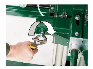
The alignment bolt can now be turned to change the angle of the bandwheel and track the blade. To move the blade more rearward on the bandwheel, this bolt will need to be turned clockwise. Alternatively, turning the bolt in the counter-clockwise direction would force the blade to run more forward on the bandwheel. Turn the bolt a 1/2 turn and re-tension the blade.
