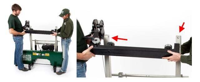
Assemble the top cross support to the square posts. Note the location and direction of the holes in the posts as shown by the arrows above. Insert and hand tighten the 4 bolts that hold the cross support to the posts. These bolts will be properly tightened properly once the head is on the track system and the head is "squared" up.
