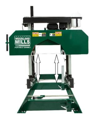
Once the head is square to the track, it can be leveled left to right to ensure the blade is sitting level to the log bunks. Using a tape measure, take a measurement from the blade to the top of the log bunk on both the left and right side. The distance should be equal on both sides. If it isn't, you will need to adjust the cable ends at the rear handle to either raise or lower one side. Refer to below step for adjustment instructions.
