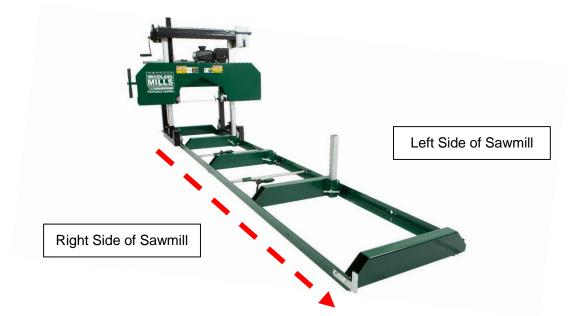
Always cut in the direction shown above. The log clamp should always be on the right side of the log and the log supports should always be on the left. Failure to cut in this direction can cause the log to come lose and possibly even cause damage or injury.
