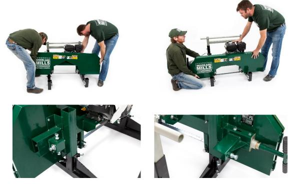
With a minimum of two people, lift and rest the head onto the carriage bases so that the head is resting on the two vertical square posts as shown in above pictures.
