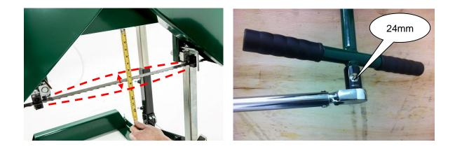
Proper blade tension is achieved when the blade deflects no more than a total of 1/8" - 1/4" up/down when it is firmly moved by hand at the center location of the blade guide blocks. Turning the blade tension "T" handle in the clockwise direction will add tension to blade. Alternatively, a 24mm socket on a torque wrench may be used to tighten the "T" handle to 35 ft-lbs torque. See above right image.
