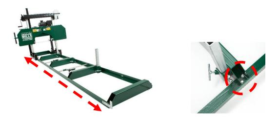
Push the saw head up and down the track system to ensure that the width of the track allows for the saw head to move freely. If it binds, the "L" rails will need to be set further or closer together to achieve a consistent width along the entire track system. Once the desired width is achieved, all nuts and bolts can be tightened to the log bunks as shown in above right image using a 14mm socket.
