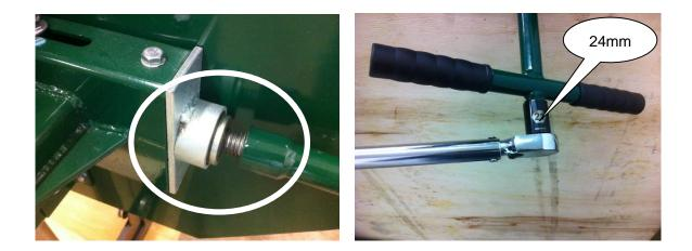
Add grease to the threads of the blade tension "T" handle and to the washer face that it meets before use. Proper blade tension is achieved with a 24mm socket on a torque wrench and is used to tighten the "T" handle to 30-35 ft-lbs torque. See above right image.
