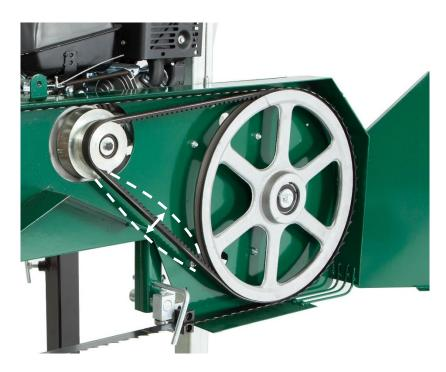
To check the belt tension, with your hand, firmly try to deflect the belt up and down. There should be no more than 1/4" of deflection in both directions (1/2" total). If the belt deflects more than this, it will need to be tightened as described below.
