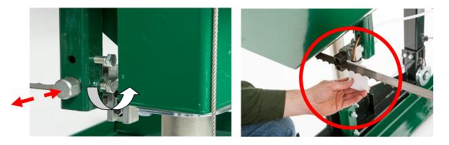
Loosen the blade guide assembly bolt with a 16mm socket. The round shaft should now be free to slide back and forth. Position it so that there is a paper width gap between the bearing and the back of blade. Tighten bolt against the flat on the shaft to secure assembly back in position.
