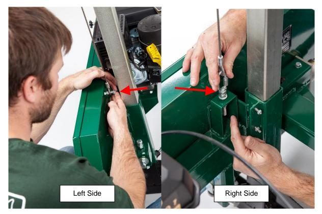
Attach cable ends to head on both sides as shown above. These are adjustable so that the blade/head assembly can be leveled to the log bunks. This will be shown and done at a later step.
