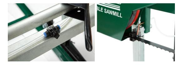
Using the bolts and nuts provided, attach the water valve to the square bar. The end of the hose can be attached to the copper pipe at the blade guide location. Insert the lube tank line through the hole in the bottom of the saw head as shown in above right image. Use a 16mm socket to secure the copper end in position. Do not over tighten or crush the copper end.
