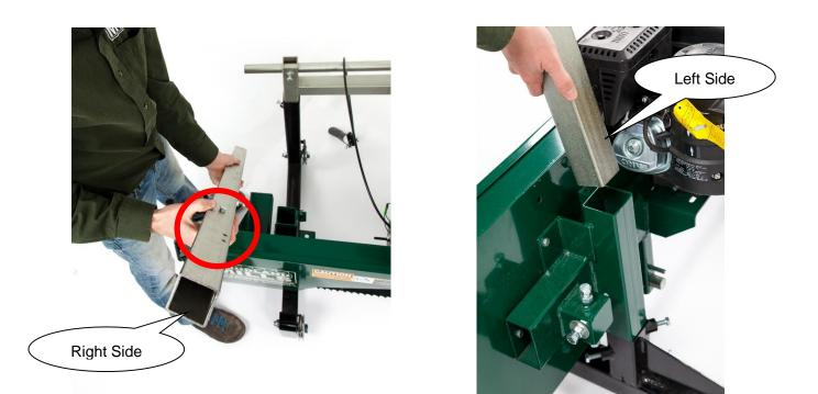
While one person is holding the head in place, have the other person insert both square posts through the head and into the carriage base on both sides. Note that the square post with the two holes and bolt circled above needs to be installed on the right side of the mill (when standing behind it). Also note on the picture on the next page the orientation of the bolt holes at the top of the square posts. These are the holes that the top cross support mounts to.
