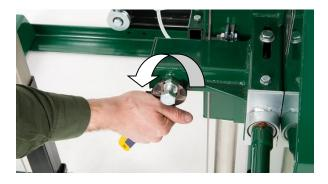
Loosen the tracking alignment locking nut with an adjustable wrench.
