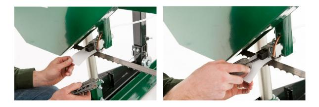
Using a piece of paper in between the blade and blade guide blocks, tighten the allen key bolts.
