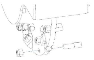
4. Install a replacement tooth and lock nut using a torque wrench set to 160 ft-lbs (215 Nm)
