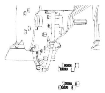
2. Slide the flywheel assembly forward and down.
