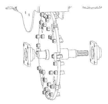
4. Installation is the reverse of removal. Tighten the lock nuts to 65 ft-lbs (88 Nm).
