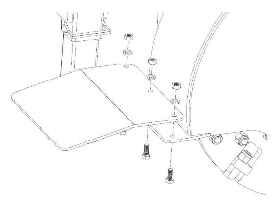
2. Install the manual tube using the 2 supplied bolts and washers.
