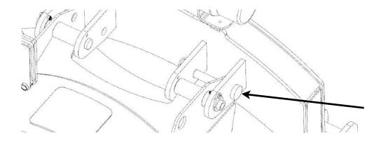
4. Move the legs up inside the tubes so they are out of the way and install the retaining pins to hold the legs in place.
