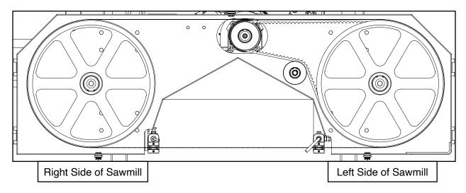
The blade should run with the same tooth to band wheel face distance on both sides: ¾" (9 mm) is ideal. The back of the blade will be just proud of the back of the band wheel at this distance and is a quicker check than using a tape measure. If an adjustment on either side is required, the below steps detail this procedure.
