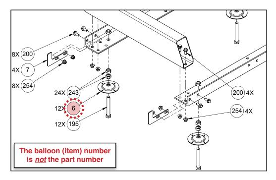
Next, turn to the *Parts List* section and locate the balloon number in the "Item" column:
