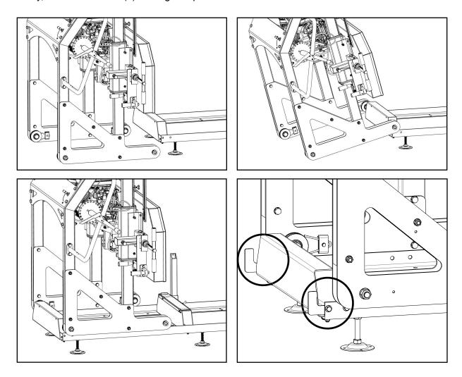
With the sawmill head assembly now resting on the track, tighten all of the bolts.
