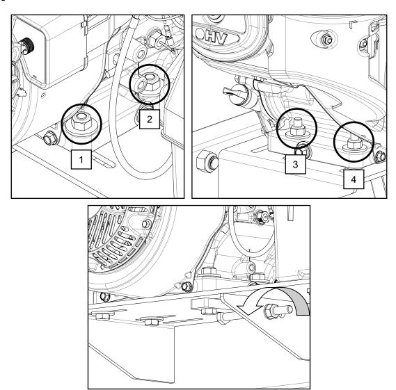
Now that the engine is free to slide on the engine mounting plate, turn the nut on the horizontal stud in the counter-clockwise direction. This will allow the engine to move and also take the tension off of the belt. The old belt can now be removed and the new belt installed. Tension the new belt and refer to the <u>BELT TENSION</u> instructions described in the <u>SAWMILL SET-UP</u> **PROCEDURES** section of the manual.
