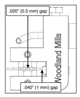
After the guide blocks and guide rollers are set, slide the adjustable blade guide in and out while noting the blade guide bearing-to-blade gap and the guide block-to-blade gap. If either of these gaps change while sliding the guide block adjustment arm, the guide angle can be adjusted via the steps on the next page.
