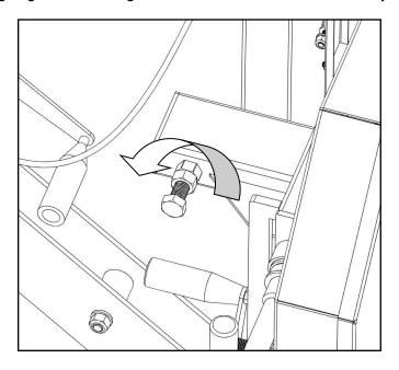
The alignment bolt can now be turned to change the angle of the band wheel and track the blade. To move the blade more rearward on the band wheel, turn this bolt clockwise. Alternatively, turning the bolt in the counter-clockwise direction will force the blade to run more forward on the band wheel. Turn the bolt ½ turn and re-tension the blade.
