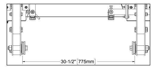
To adjust the width of the wheels, washers may be added or removed from each wheel to ensure a distance of 30.5" (775 mm) is achieved as shown below.
