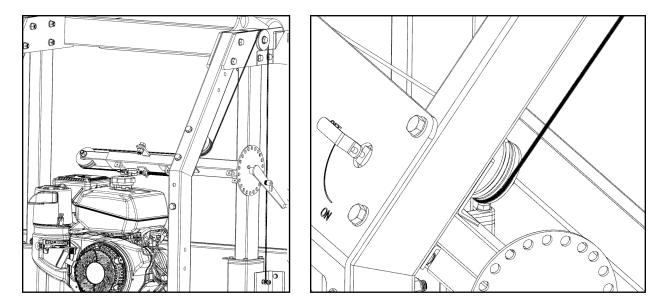
Be sure to securely tighten the oval chain link with a wrench after the cable loop ends have been attached.
