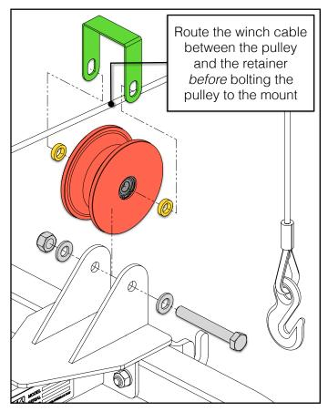
Ensure the spacers are between the pulley bearings and the *inside* faces of the mount flanges.
