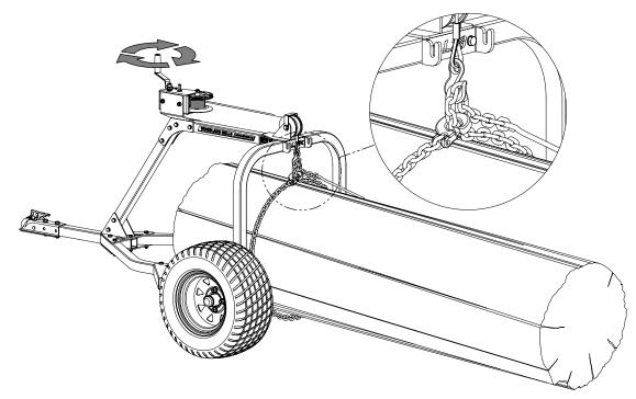
4. Hook the loose end of the chain onto the rear arch hook.
