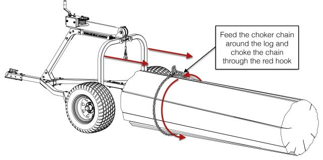
2. Hook the loose end of the chain onto the winch cable grab hook.
