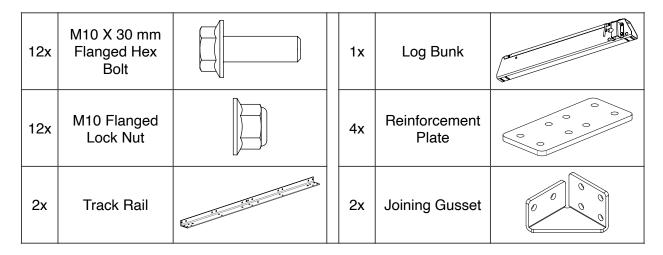
Track components listed in these tables are *not* included with the trailer package, namely track rails, reinforcement plates, bunks, and carriage stops. These components are found in the sawmill crate. If the trailer was purchased for an existing sawmill (i.e. the sawmill is currently assembled), the track will need to be disassembled prior to building the trailer.
