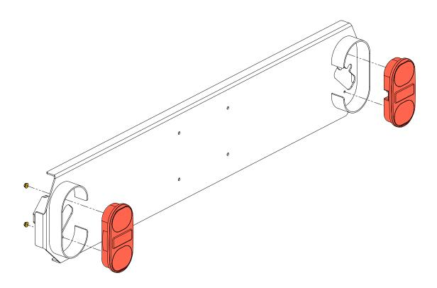
\*\*Note: Tail lights (North America and Europe) and side lights (North America only) are integral to the wire harness. They are shown exploded for assembly clarity.\*\*
