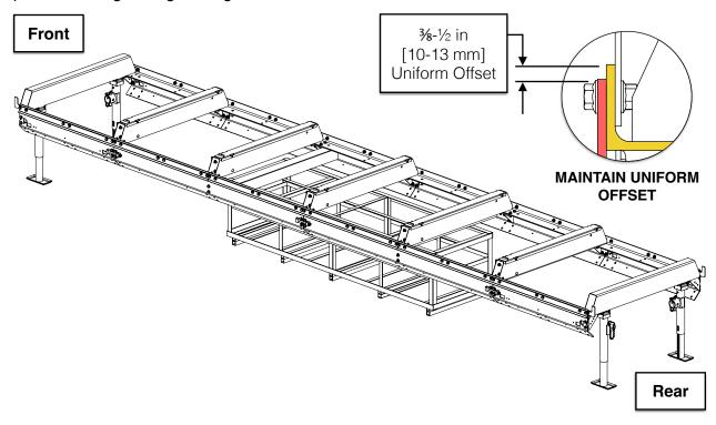
While maintaining a uniform side plate-to-rail offset, torque the remaining bolts per the table in section, **BOLT TORQUE SPECIFICATIONS**, starting from the centre and working towards the outer ends. Ensure the track is straight, level, and square during this procedure.
