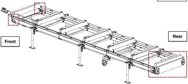
Secure tail lights to the taillight bracket using M5 flanged lock nuts before mounting taillight bracket to trailer.
