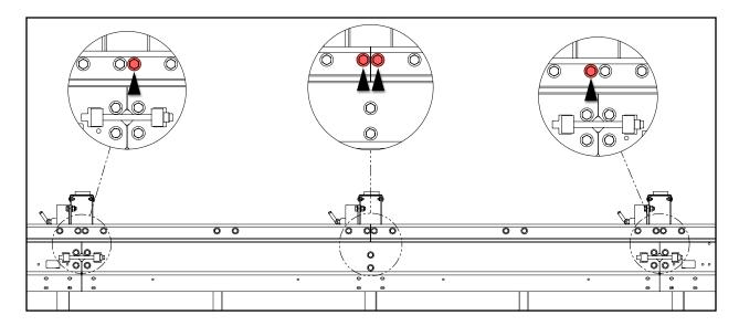
With the long side plate secured in place, note the gaps (if any) between the short side plates and the long side plates.
