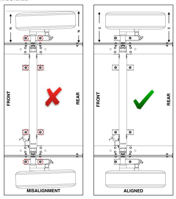
If the wheels are parallel, tighten the axle bolts to the **specified torque** and proceed to the next section. However, if the wheels are *not* parallel, loosen the four (4) M12 bolts on the affected axle(s). Rotate the axle assembly and wheel until the wheels are parallel. Then tighten the axle bolts to the **specified torque**.
