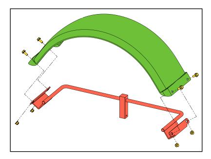
Slide the post on the fender bracket into the sleeve on the axle mount and insert the locking pin through the hole located at the bottom of the fender bracket post. Secure the fender/fender bracket sub-assembly using the M10 X 30 mm knob by threading it into the axle mount until tight.
