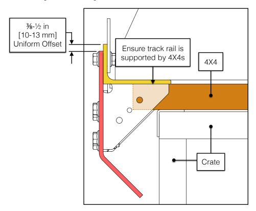
If the offset is not uniform, ensure the track is sitting on the 4X4s and not the crate. The side plates need to hang from the rails unobstructed, with only the force of gravity pulling them down.
