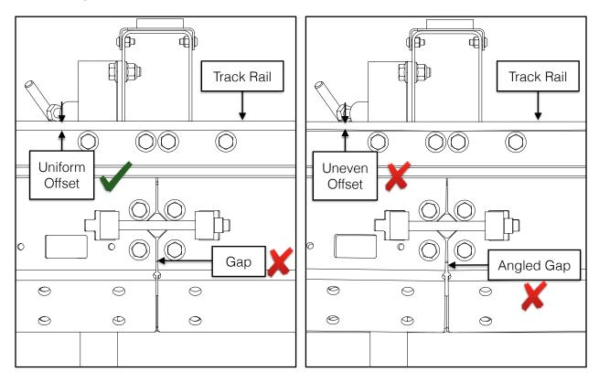
If there are gaps, they can be closed by tightening the M10 X 120 mm Socket Head Cap Screw. Tighten all four (4) M10 X 120 mm Socket Head Cap Screws to close the gaps.
