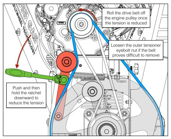
5. With the drive belt removed, remove the outer hex nut from the belt tensioner eyebolt.
