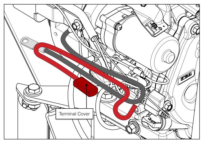
The positive cable (red) ships with a cover on the terminal. If the wood chipper will be set up to use only the recoil start (i.e. the electric start will not be utilized), keep the cover on the terminal. However, if the electric start *will* be utilized, remove the cover and proceed with the remainder of the battery installation.
