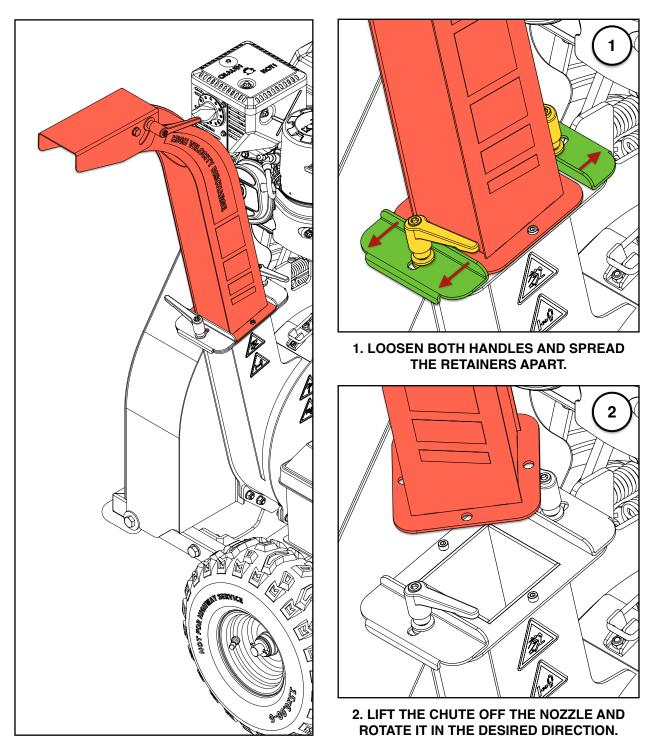
To rotate the discharge chute in an alternate direction, follow these steps:
