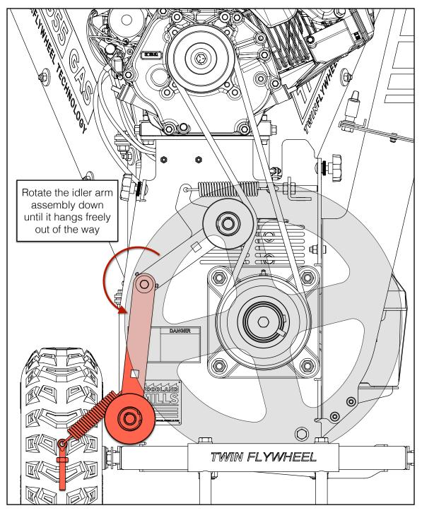
With the idler out of the way, the impeller belt tensioner arm is now accessible.
