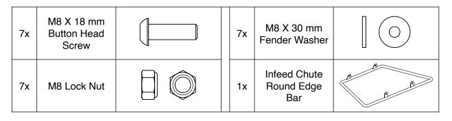
Position the lower tabs of the round edge bar *under* the bottom panel and the upper tabs *over* the top panel. Pivot the top chute panel slightly if necessary. Secure the round edge bar using three (3) M8 X 18 mm button head screws, three (3) M8 X 30 mm fender washers, and three (3) M8 lock nuts. **Do not install any hardware through the upper-left tab**.
