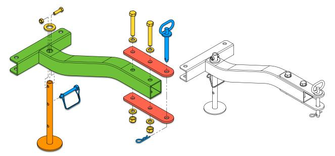
To secure the tow bar assembly to the base, use two (2) M12 X 70 mm hex bolts, four (4) M12 flat washers, and two (2) M12 lock nuts. Fully tighten the hardware.
