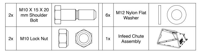
With the assistance of a second person supporting the infeed chute assembly, assemble the chute to the wood chipper using two (2) M10 X 15 X 20 mm shoulder bolts, six (6) M12 nylon flat washers, and two (2) M10 lock nuts. Tighten the hardware ensuring the chute swings freely.
