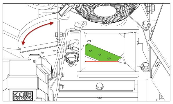
Continue to rotate the flywheel to check the remaining two blades relative to the bed plate, noting which blade is closest. Use the blade with the closest gap when setting the bed plate gap.
