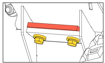
Place the short bent end of the bed plate gap tool between the bed plate and the blade and then push the bed plate against the tool. Move the tool left-to-right along the bed plate's length to ensure the gap is uniform along the edge of the blade.
