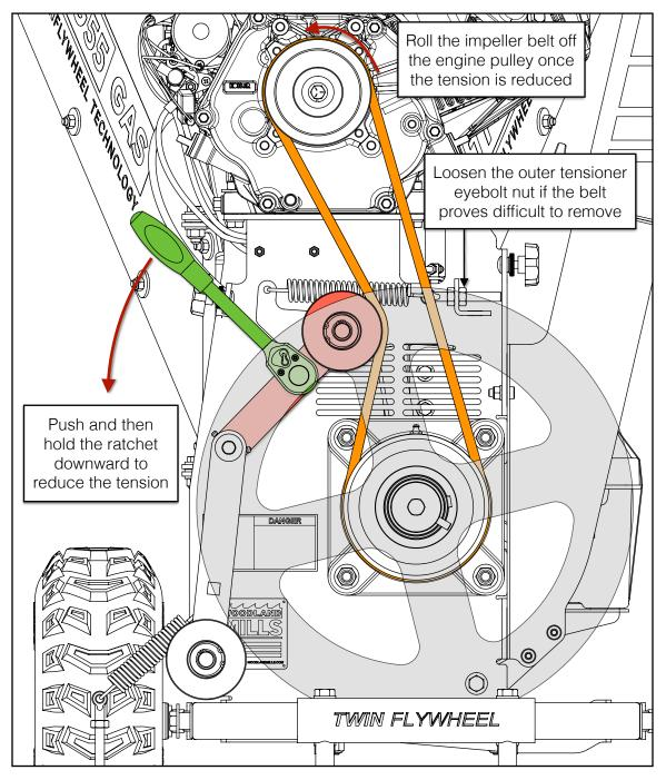
While it is not necessary to remove the tensioner eyebolt from its mounting flange, the outer nut can be loosened to assist with removing the belt if it still proves difficult.
