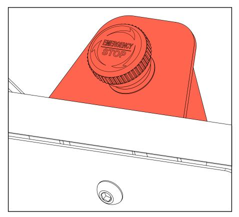
To reset the switch, twist the red button in the direction indicated by the arrows on its face until it "pops" back up. Ensure the engine throttle is set to "tortoise" before restarting.
