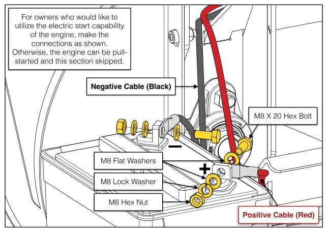
Once the connections are made, set the battery box lid on top ensuring the battery cables route down and out the openings in the side. Use the included strap to secure the top and bottom halves of the battery box.
