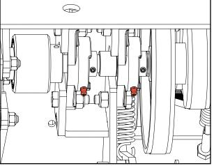
Pump Shaft Bearings (2x Underside)
