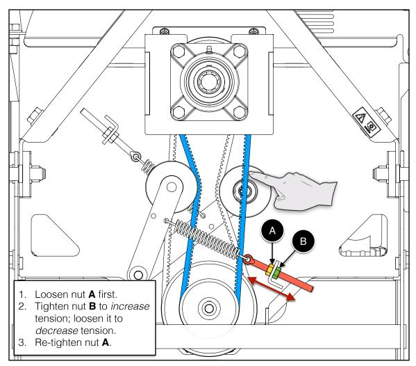
Adjusting Hydraulic Pump Belt Tension [Connecting rod removed from image for clarity]
