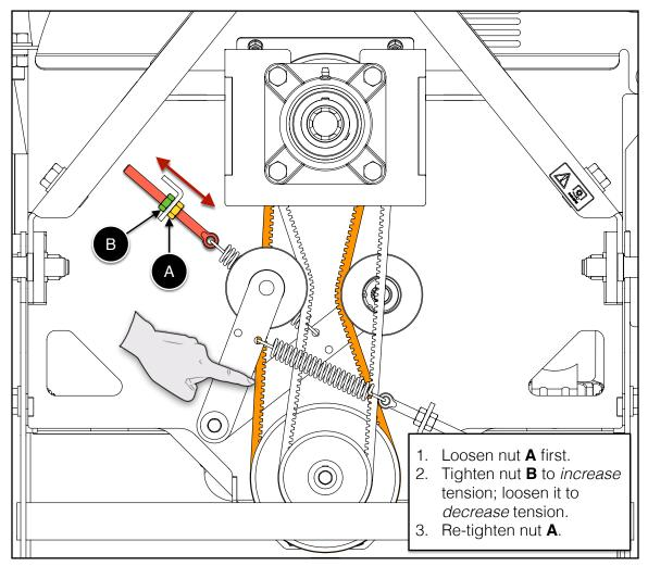
Adjusting Paddle Flywheel Belt Tension [Connecting rod and pump belt & tensioner removed from image for clarity]
