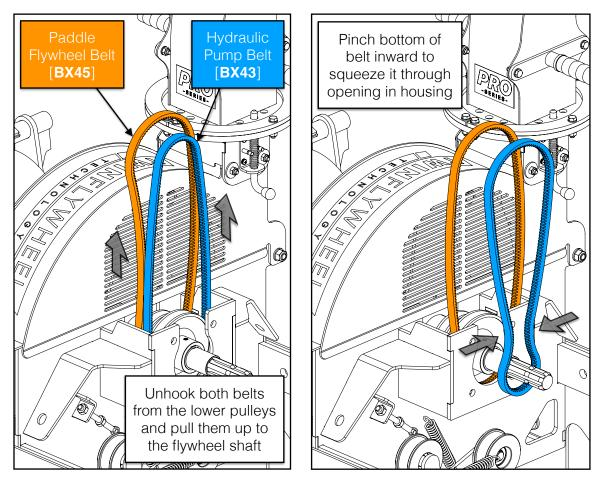
9. Reverse the steps to install new belts. Remember to install the paddle flywheel belt (rear) first before installing the hydraulic pump belt (front).
