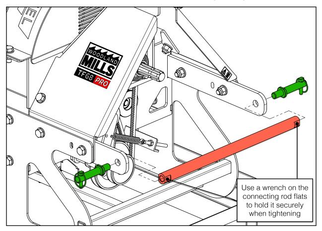
With the connecting rod tight, now fully tighten all the hardware for the lower hitch arms from the previous step.
