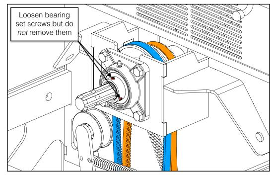
6. Loosen-do not remove-the two (2) M8 set screws on the rear bearing's collar.
