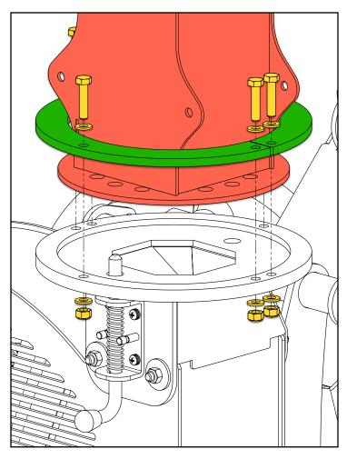
Assemble the handles—one on each side of the discharge chute.
