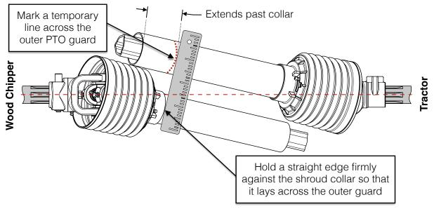
Measure 1 in [25 mm] past the marked line to the guard tube end to determine the trim length. This is the "**Trim Length**" by which the PTO shaft needs to be trimmed. Proceed to Step 5.
