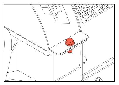
3. With the flywheel exposed, manually rotate it so that one of the four (4) locking holes in the flywheel (near the front of the blade) approximately lines up with the flywheel lock pin at the rear of the housing. Remove the round locking pin from the flywheel lock pin and flip the flywheel lock pin around 180°, passing it through the housing and into the locking hole in the flywheel. Reinstall the smaller locking pin to the flywheel lock pin.
