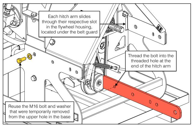
Use two (2) M16 X 55 mm bolts, four (4) M16 flat washers, and two (2) M16 lock nuts to secure the arm. Only snug the hardware, do not fully tighten them until instructed in a later step.
