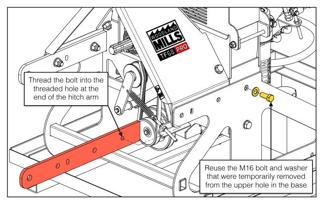
Use two (2) M16 X 55 mm bolts, four (4) M16 flat washers, and two (2) M16 lock nuts to secure the arm. Only snug the hardware, do not fully tighten them until instructed in a later step.
