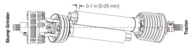
*Scenario 3.* If the guard tube end extends past the shroud collar, hold a straight edge firmly against the shroud collar so that it lays across the outer guard. Mark the position on the outer guard.
