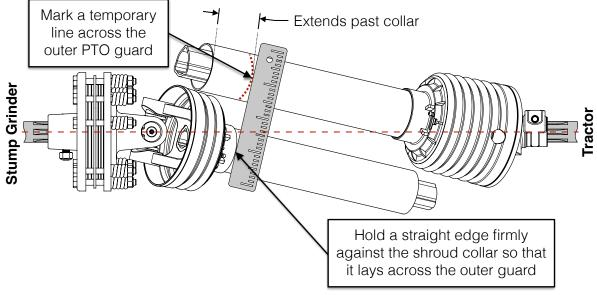
Measure 1 in [25 mm] past the marked line to the guard tube end to determine the trim length. This is the "**Trim Length**" by which the PTO shaft needs to be trimmed. Proceed to Step 5.
