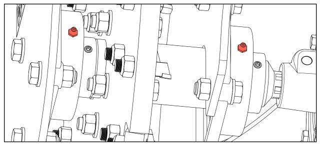
Flywheel Shaft Bearings (Underside of Flywheel Housing)
