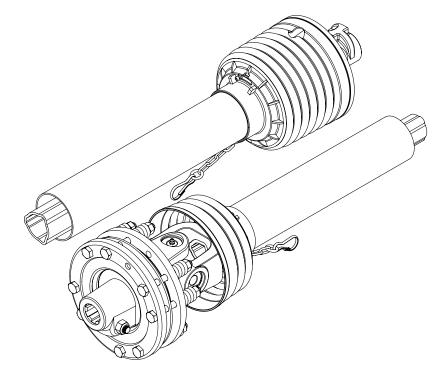
2. Use a slotted screwdriver to remove the red bearing plug from the shroud.
