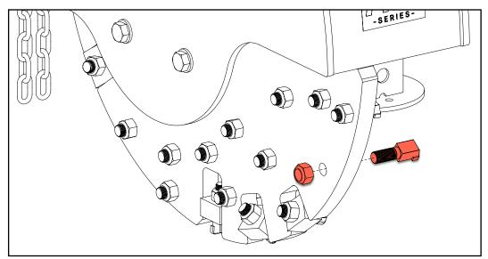
Install the replacement tooth and lock nut using a torque wrench set to 160 ft•lb [215 N•m]. Refer to section <u>FLYWHEEL TOOTH TORQUING</u> for more detail.
