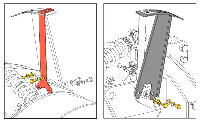
With all the fasteners tight, the "GO" text should be centred in the indicator view window.
