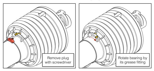
3. Rotate the guard bearing by its grease fitting until it stops at the opposite side of the slot.
