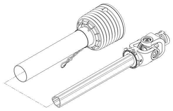
5. Stretch the guard bearing apart at its split and pull it out of the groove in the yoke collar.
