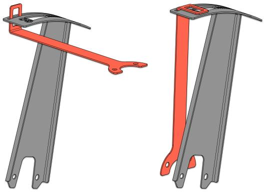
Holding the indicator perpendicular to the gauge, insert the view window tab of the indicator up though the bottom of the long slot in the gauge. Then rotate the indicator back down until they are parallel with each other.
