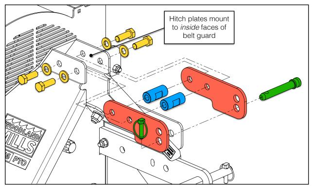
When tightening the hardware, hold the bushings still with an adjustable or 15/16 in [24 mm] wrench and turn the hex bolts with a second wrench or ratchet. Fully tighten all the hardware.
