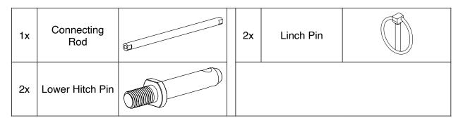
Position the connecting rod between the two (2) lower hitch arms and then thread one (1) lower hitch pin into each end, securing it to the arms. The flats at both ends of the connecting rod will accommodate a  $1-\frac{1}{8}$  in [28 mm] wrench to prevent it from rotating when tightened.
