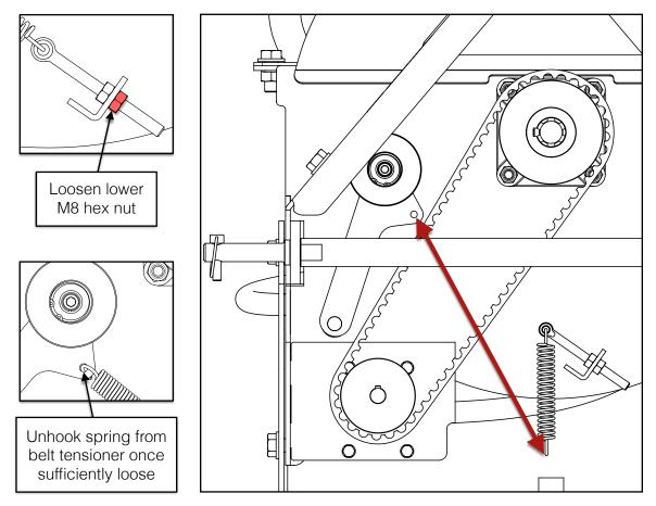
Install the new belt around the pulleys first and then reinstall the spring. Re-tension the spring by tightening the lower M8 hex nut on the eyebolt. Refer to the previous section, <u>ADJUSTING THE HYDRAULIC PUMP BELT TENSION</u>, for instructions on how to properly re-tension the belt.
