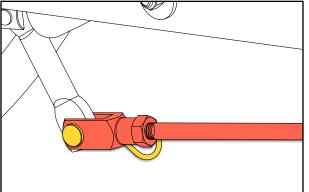
Once the linkage has been assembled, ensure both M10 jam nuts are tight.
