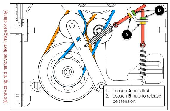
5. Unhook the extension springs from the eyebolts and allow the belt tension arms to rotate downward until they come to rest.
