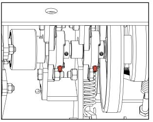
Pump Shaft Bearings (2x Underside)
