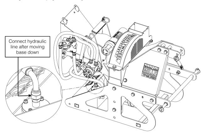
With the base secure and hydraulic line connected, slide the crate skid out from under the wood chipper and discard it.
