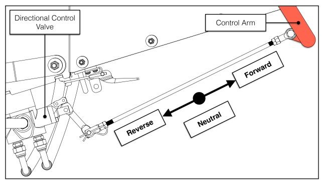
To change the speed of the infeed roller, place the red control arm in the *neutral* position. This stops the infeed roller from rotating. The speed control valve can now be moved to the desired position/speed. Reengage the infeed roller via the control arm.
