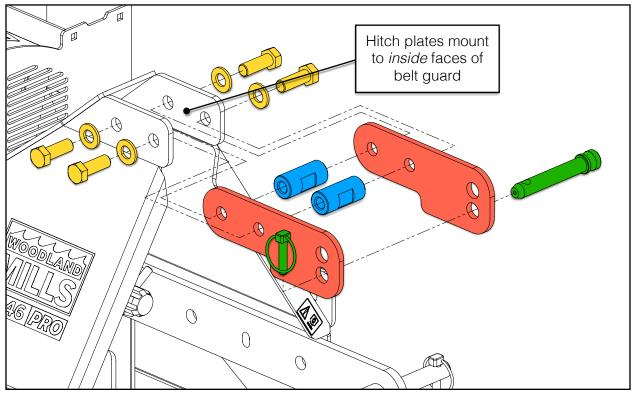
When tightening the hardware, hold the bushings still with an adjustable or 15/16 in [24 mm] wrench and turn the hex bolts with a second wrench or ratchet. Fully tighten all the hardware.
