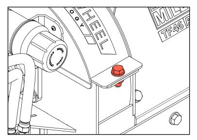
3. With the flywheel exposed, manually rotate it so that one of the four (4) locking holes in the flywheel (near the front of the blade) approximately lines up with the flywheel lock pin at the rear of the housing. Remove the small locking pin from the flywheel lock pin and flip the flywheel lock pin around 180°, passing it through the housing and into the locking hole in the flywheel. Reinstall the smaller locking pin to the flywheel lock pin.
