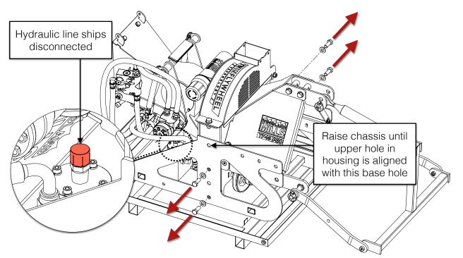
With the base separated, use the tractor's 3-point hitch to raise the chipper chassis up until the uppermost threaded holes in the side of the flywheel housing are aligned with the uppermost base holes.
