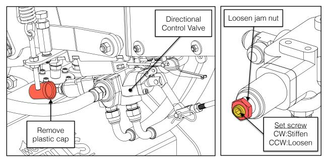
Loosen the jam nut with a 22 mm [ $\frac{7}{8}$  in] wrench. Use a 6 mm hex key and turn the set screw *clockwise to stiffen* the movement of the arm, *counter-clockwise to loosen* it. Tighten the jam nut and replace the cap after the control arm movement feels satisfactory.
