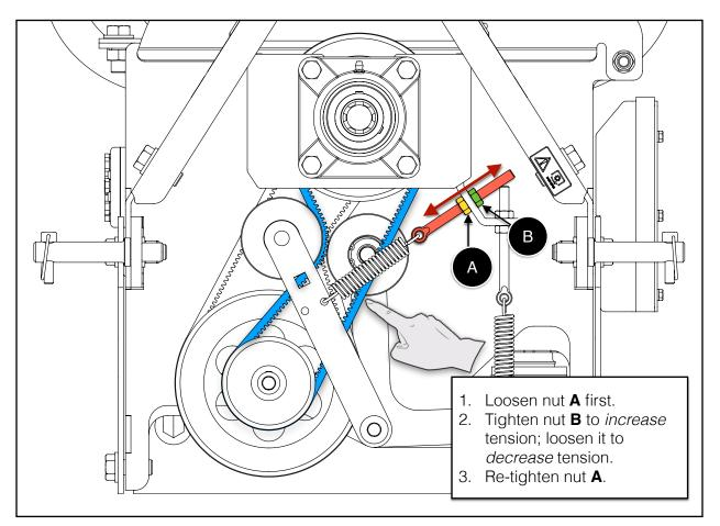
Adjusting Hydraulic Pump Belt Tension [Connecting rod removed from image for clarity]
