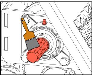
Rear Flywheel Shaft Bearing and Flywheel Shaft Spline
