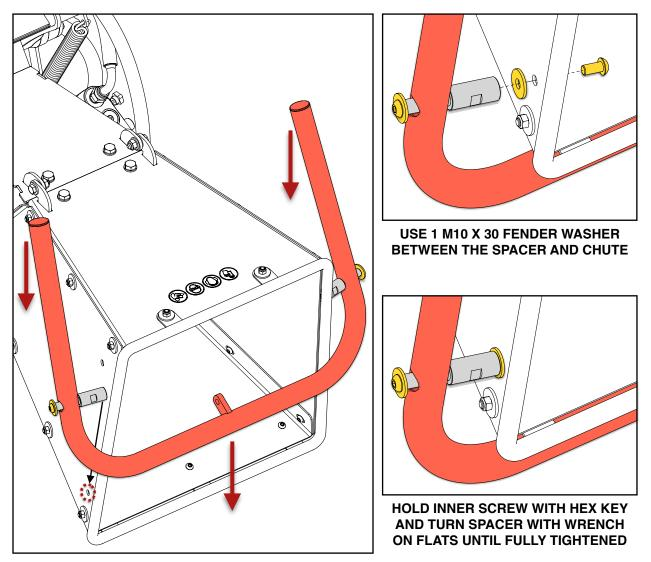
With the spacers aligned with the holes in the infeed chute side panels, place one (1) M10 X 30 mm fender washer between the spacer and side panel, and then secure it with one (1) M10 X 20 mm button head screw from inside the infeed chute. Repeat for the other side.
