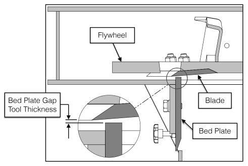
Place the bed plate gap tool between the bed plate and blade. Verify that the gap is consistent vertically from the top of the bed plate to the bottom.
