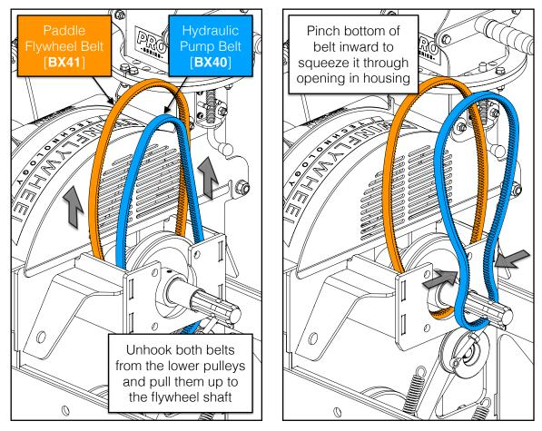
9. Reverse the steps to install new belts. Remember to install the paddle flywheel belt (rear) first before installing the hydraulic pump belt (front).
