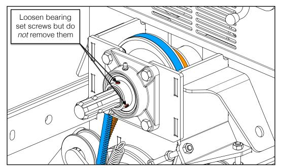
6. Loosen-do not remove-the two (2) M8 set screws on the rear bearing's collar.
