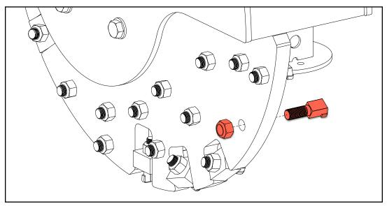
Install the replacement tooth and lock nut using a torque wrench set to 160 ft•lb [215 N•m]. Refer to section, *FLYWHEEL TOOTH TORQUING*, for more detail.
