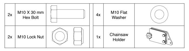
Using two (2) M10 X 30 mm bolts, four (4) M10 flat washers, and two (2) M10 lock nuts, assemble the chainsaw holder assembly to the flywheel housing. Fully tighten the hardware.
