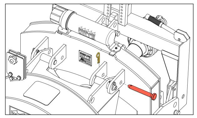
4. Remove the cotter pin from the stabilizer pin and then slide it out from the back frame hinge:
