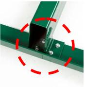
Push the saw head up and down the track system to ensure that the width of the track allows for the saw head to move freely. If it binds, the "L" rails will need to be set further or closer together to achieve a consistent width along the entire track system. Once the desired width is achieved, all nuts and bolts can be tightened to the log bunks as shown in above left image using a 16mm socket.
