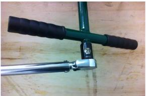
Proper blade tension is achieved when the blade deflects no more than a total of 1/8" - 1/4" up/down when it is firmly moved by hand at the center location of the blade guide blocks. Turning the blade tension "T" handle in the clockwise direction will add tension to blade. Alternatively, a 21mm socket on a torque wrench may be used to tighten the "T" handle to 60 ft-lbs torque. See above right image.
