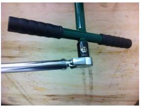
Add waterproof grease to the threads of the blade tension "T" handle and to the washer face that it meets before use. Proper blade tension is achieved when the blade deflects no more than a total of 1/8" - 1/4" up/down. Alternatively, a 21mm socket on a torque wrench may be used to tighten the "T" handle to 60 ft-lbs torque. See above right image.
