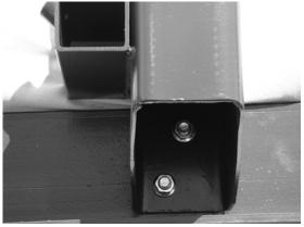
Attach track cross supports to "L" channel with the provided nuts & bolts. Ensure to only hand tighten at this stage. The bolts will be fully tightened once the head assembly is free to roll on the tracks and provide the correct track width.
