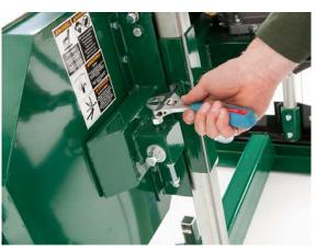
To adjust the left side of the sawmill, again start by taking the tension off of the blade by turning the "T" handle one turn in the counter-clockwise direction. Using a 16mm wrench, loosen the "vertical nut" a ½ turn. Do the same on the "bottom vertical nut". Next, loosen both "vertical bolts" a ½ turn. This will take the clamping force off of the bandwheel shaft caused by these two bolts and allow it to move freely in the following steps.
