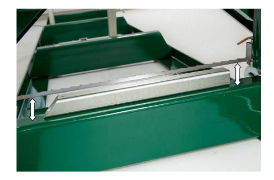
Using a tape measure, take a measurement from the blade to the top of the log bunk on both the left and right side. The distance should be equal on both sides. If it isn't, you will need to adjust the cable ends at the rear handle to either raise or lower one side. Refer to below step for adjustment instructions.
