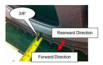
The blade should run with the same tooth to bandwheel face distance on both sides. 3/8" is ideal. Measure the distance from the tip of the blade tooth to the front face of the bandwheel on both sides. If an adjustment on either side is required, the below steps will detail this procedure.
