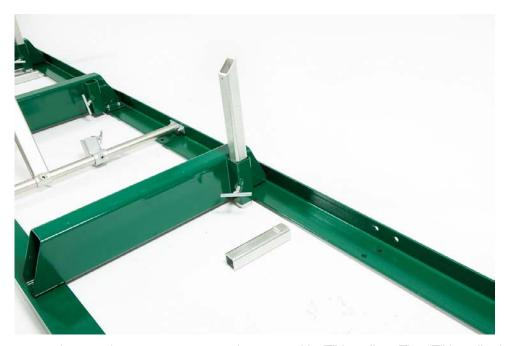
Insert log supports into track cross supports and secure with "T" handles. The "T" handle threads should be coated with waterproof grease. The sawmill includes two sets of log supports – a short set and a long set. The longer set is ideal for larger logs and the shorter set is ideal for small logs and square cants.
