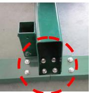
Push the saw head up and down the track system to ensure that the width of the track allows for the saw head to move freely. If it binds, the "L" rails will need to be set further or closer together to achieve a consistent width along the entire track system. Once the desired width is achieved, all nuts and bolts can be tightened to the log bunks as shown in above right image using a 16mm socket.
