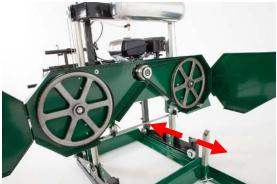
Remove the tension in the blade by turning the "T" handle in the counter-clockwise direction and then open the blade guard cover. The blade should now be loose and free to pull straight out the front. The new blade can now be installed, guards closed and proper blade tension set.
