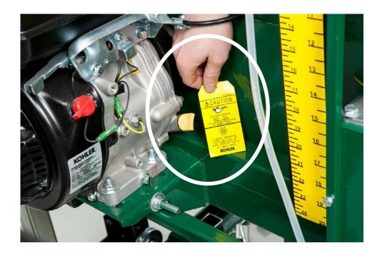
Refer to the engine manual before using your sawmill. Please note that the engine does not contain any gasoline or engine oil when it is shipped. Furthermore, the engine is equipped with an oil alert system, meaning that if the crankcase oil level is low or empty, the power is cut to the spark plug and it will not start.
