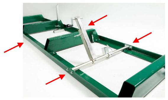
Attach log dog assembly to track as shown above with the 4 nuts and bolts provided. Note that there are various locations along the track where this assembly can be bolted. Depending on how many track sections are being used, select a log clamp position that will secure the log firmly against the log supports.
