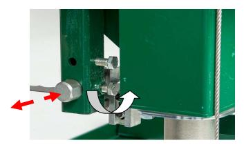
Loosen the blade guide assembly bolt with a 16mm socket. The round shaft should now be free to slide rearward and out of the way. Perform this step on both guide assemblies. This will ensure that the guide bearings do not influence tracking of the blade while adjusting.
