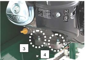
To change the drive side belt, loosen the four bolts that secure the engine to the engine mount using a 16mm wrench.
