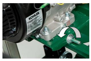
Now that the engine is free to slide on the engine mounting plate, turn the 16mm nut on the horizontal stud in the counter-clockwise direction. This will allow the engine to move and will also take the tension off of the belt. The old belt can be removed and the new belt can be installed. Tension the new belt and refer to the <u>BELT TENSION</u> instructions described in the sawmill set up section of the manual.
