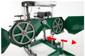
Remove the tension in the blade by turning the "T" handle in the counter-clockwise direction and then open the blade guard cover. The blade should now be loose and free to pull straight out the front.
