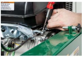
Install the throttle handle to the round bar as shown in above left image. With the throttle lever in the idle position/fully open, pull the cable tight at the engine and tighten the screw to hold it in place. This will take all of the slack out of the cable.
