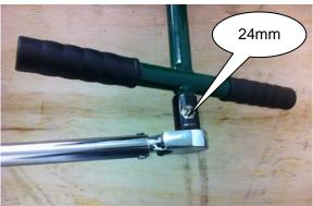
Proper blade tension is achieved when the blade deflects no more than a total of 1/8" - 1/4" up/down when it is firmly moved by hand at the center location of the blade guide blocks. Turning the blade tension "T" handle in the clockwise direction will add tension to blade. Alternatively, a 24mm socket on a torque wrench may be used to tighten the "T" handle to 55 ft-lbs torque. See above right image.
