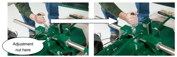
Lock the cam handles on both the round and square post to prevent the head from moving when it is stood up in the coming steps. Ensure that when activating the cam handles, the clamps securely lock on the round and square vertical post. If they don't, a 13mm wrench will need to be used to tighten the adjustment nut. This will allow the clamps to lock on the post better.
