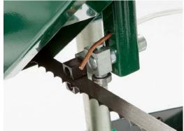
Insert the lube tank line through the hole in the bottom of the saw head as shown above. Use a 16mm socket to secure the copper end in position. Do not over tighten or crush the copper end.
