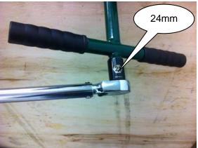
Add waterproof grease to the threads of the blade tension "T" handle and to the washer face that it meets before use. Proper blade tension is achieved when the blade deflects no more than a total of 1/8" - 1/4" up/down. Alternatively, a 24mm socket on a torque wrench may be used to tighten the "T" handle to 55 ft-lbs torque. See above right image.
