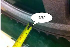
Re-tension the blade by turning the "T" handle a full turn in the clockwise direction. Wearing gloves, spin the bandwheel with your hand and observe how the blade has changed tracking. Measure the distance again and repeat the above step to further compensate if required. The ideal measurement is 3/8".
