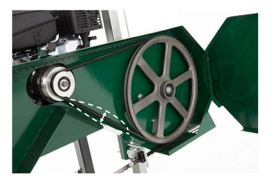
To check the belt tension, with your hand, firmly try to deflect the belt up and down. There should be no more than 1/4" of deflection in both directions (1/2" total). If the belt deflects more than this, it will need to be tightened as described below.
