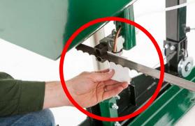
Loosen the blade guide assembly bolt with a 16mm socket. The round shaft should now be free to slide back and forth. Position it so that there is a paper width gap between the bearing and the back of blade. Tighten bolt against the flat on the shaft to secure assembly back in position.
