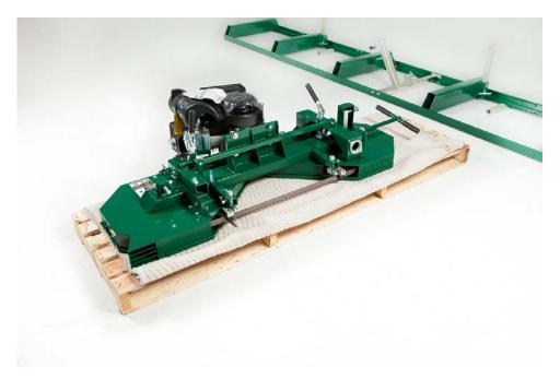
Place a moving blanket on the shipping pallet that the sawmill crate was strapped to. The blanket will prevent the blade guard covers from becoming scratched. Using a **minimum of two people** or a mechanical advantage system, remove the head assembly from the sawmill crate and place face down on the blanket. The head assembly is very heavy, proper technique must be used to avoid injury or damage.
