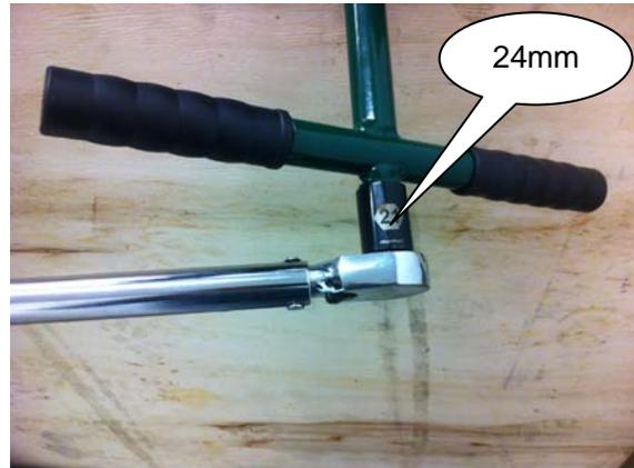
Add waterproof grease to the threads of the blade tension "T" handle and to the washer face that it meets before use. Proper blade tension is achieved when the blade deflects no more than a total of 1/8" - 1/4" up/down. Alternatively, a 24mm socket on a torque wrench may be used to tighten the "T" handle to 35 ft-lbs torque. See above right image.
