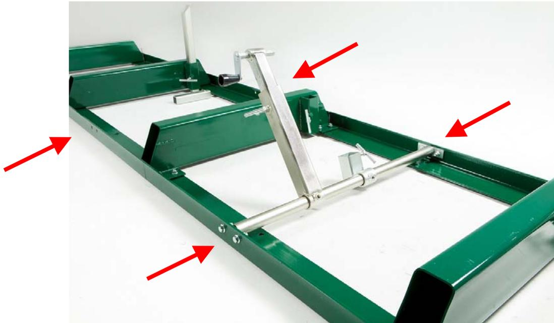
Attach log dog assembly to track as shown above with the 4 nuts and bolts provided. Note that there are various locations along the track where this assembly can be bolted. Depending on how many track sections are being used, select a log clamp position that will secure the log firmly against the log supports.
