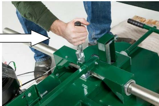
Lock the cam handles on both the round and square post to prevent the head from moving when it is stood up in the coming steps. Ensure that when activating the cam handles, the clamps securely lock on the round and square vertical post. If they don't, a 13mm wrench will need to be used to tighten the adjustment nut. This will allow the clamps to lock on the post better.
