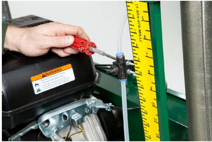
Install the lube tank line to the bracket on the scale by using a Phillips head screw driver and adjustable wrench.
