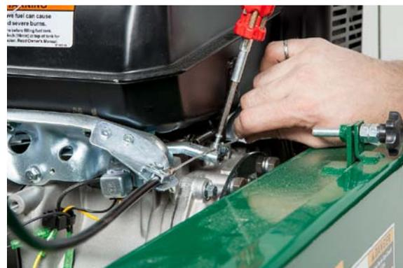
Install the throttle handle to the round bar as shown in above left image. With the throttle lever in the idle position/fully open, pull the cable tight at the engine and tighten the screw to hold it in place. This will take all of the slack out of the cable.
