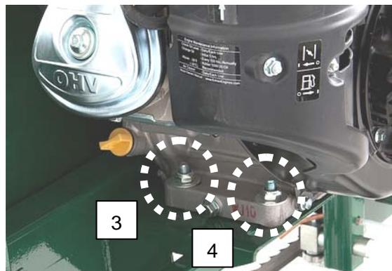
To tighten the drive belt, start by loosening the four bolts that secure the engine to the engine mount using a 16mm wrench.
