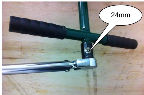
Proper blade tension is achieved when the blade deflects no more than a total of 1/8" - 1/4" up/down when it is firmly moved by hand at the center location of the blade guide blocks. Turning the blade tension "T" handle in the clockwise direction will add tension to blade. Alternatively, a 24mm socket on a torque wrench may be used to tighten the "T" handle to 35 ft-lbs torque. See above right image.
