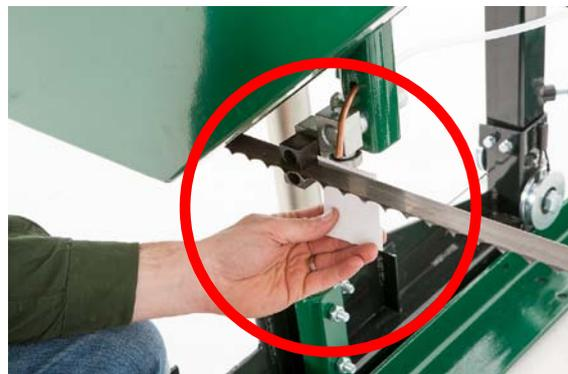
Loosen the blade guide assembly bolt with a 16mm socket. The round shaft should now be free to slide back and forth. Position it so that there is a paper width gap between the bearing and the back of blade. Tighten bolt against the flat on the shaft to secure assembly back in position.
