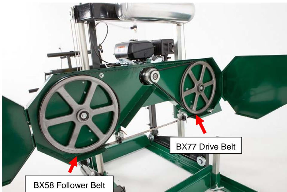
There are two rubber “V” belts on the sawmill and they should be replaced as a set. It is not advised to replace individual belts separately. It is recommended to use a BX77 cogged belt for the drive side and a BX58 follower belt.
