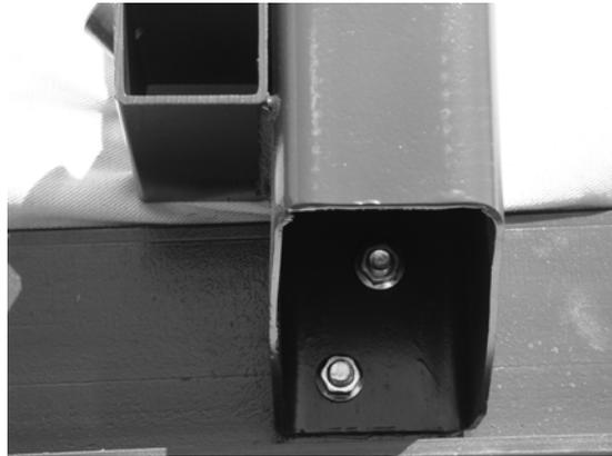
Attach track cross supports to “L” channel with the provided nuts & bolts. The joining plate is used at the seam joint to join the two sections together (shown in top right image). Ensure to only hand tighten at this stage. The bolts will be fully tightened once the head assembly is free to roll on the tracks and provide the correct track width.
