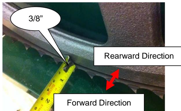
The blade should run with the same tooth to bandwheel face distance on both sides. 3/8" is ideal. Measure the distance from the tip of the blade tooth to the front face of the bandwheel on both sides. If an adjustment on either side is required, the below steps will detail this procedure.
