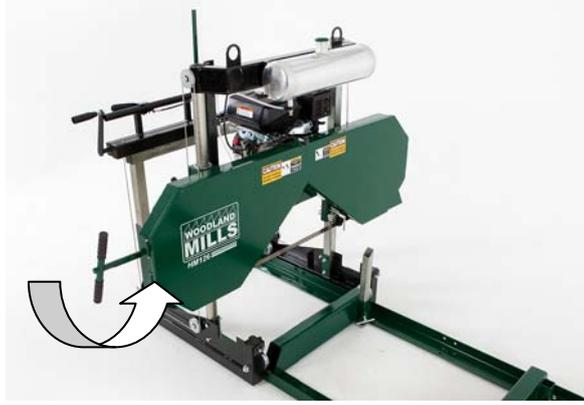
Take some tension off of the blade by turning the “T” handle in the counter-clockwise direction one full turn from full tension position.
