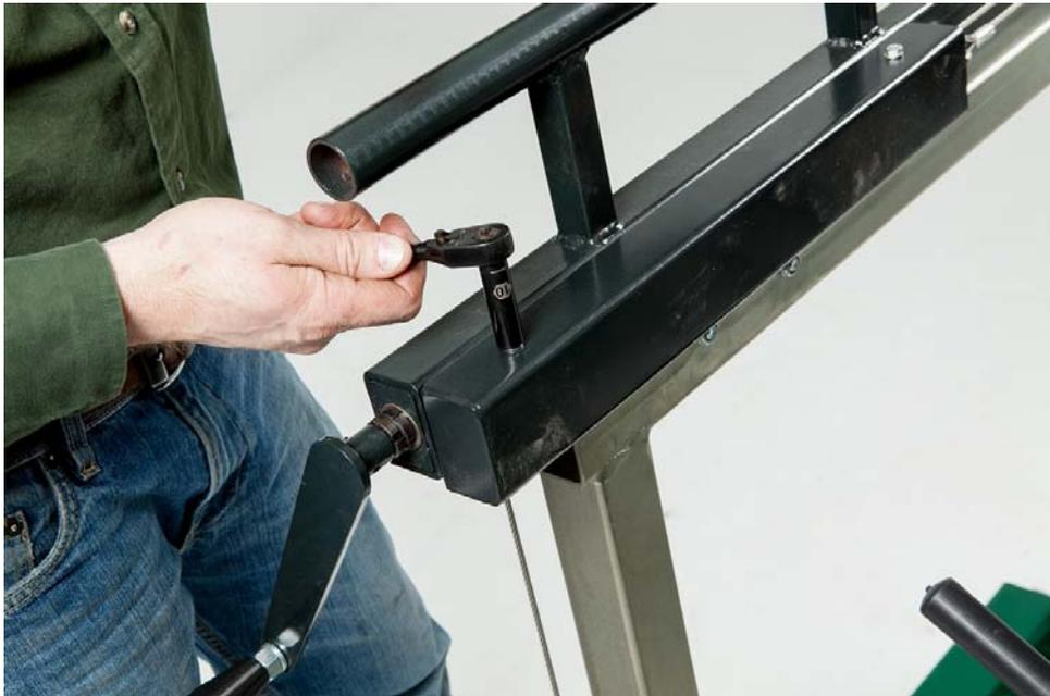
Install the cover and tighten the two bolts on the top and two on the bottom to secure it in place. Use a 10mm socket for all four bolts.
