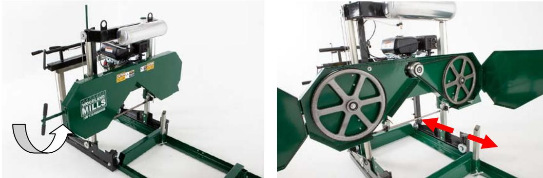
Remove the tension in the blade by turning the “T” handle in the counter-clockwise direction and then open the blade guard cover. The blade should now be loose and free to pull straight out the front. The new blade can now be installed, guards closed and proper blade tension set.
