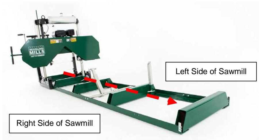
Always cut in the direction shown above. The log clamp should always be on the right side of the log and the log supports should always be on the left. Failure to cut in this direction can cause the log to come loose and possibly even cause damage or injury.
