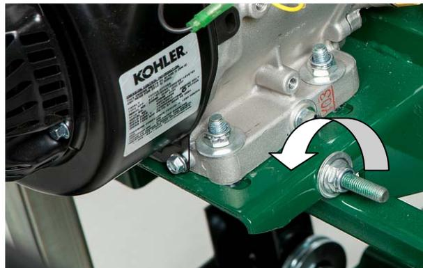
Now that the engine is free to slide on the engine mounting plate, turn the 16mm nut on the horizontal stud in the counter-clockwise direction. This will allow the engine to move and will also take the tension off of the belt. The old belt can be removed and the new belt can be installed. Tension the new belt and refer to the **BELT TENSION** instructions described in the sawmill set up section of the manual.
