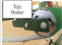
22. The top half can now be latched to the bottom half as shown below. Once latched in place, one person can begin to lift the conveyor up so another person can slide the support leg in place and latch the chain.
