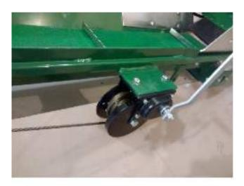
26. Remove the pulley on the operator side of the conveyor, feed the cable through and reinstall the pulley.
