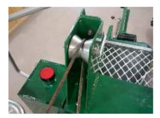
28. Attach the hook to the hook attachment point on the conveyor.
