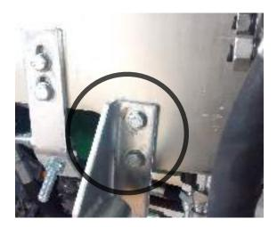
11. Install the piston between the chainsaw bar handle and the back plate as shown below. Do not over tighten the bolt at the handle as is needs to be loose to enable it to rotate smoothly.
