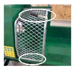
14. Install the larger cage by sliding the pipe into the hole and resting the other side on the bracket. Use the supplied bolt and nut to keep the bar it in place so it can freely rotate open and closed.
