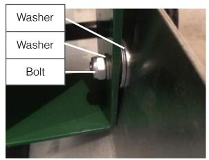
21. The top half of the conveyor can now be installed to the bottom half by bolting it at the seam using the hardware shown below. Be sure to install one of the washers in between the top and bottom conveyor. The nut should be left loose so that the bolts act as a hinge and allow the conveyor system to fold in half. Also, be sure that the conveyor is looped around the top roller.
