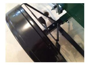
5. The four lug nuts of each wheel should be torque to 90 ft-lbs.
