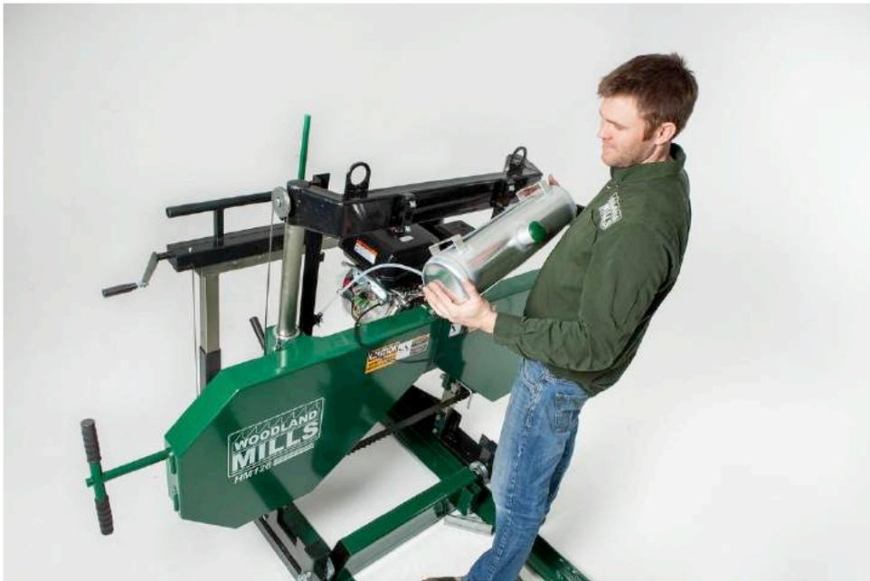
Install the aluminum lube tank to the top cross support using the four nuts and bolts provided.
