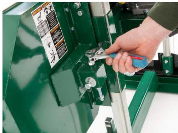
To adjust the left side of the sawmill, again start by taking the tension off of the blade by turning the "T" handle one turn in the counter-clockwise direction. Using a 17mm wrench, loosen the "**vertical nut**" a 1/2 turn. Do the same on the "**bottom vertical nut**". Next, loosen both "**vertical bolts**" a 1/2 turn. This will take the clamping force off of the bandwheel shaft caused by these two bolts and allow it to move freely in the following steps.
