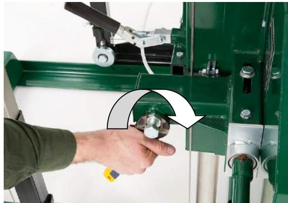
Once satisfied with the measurement, tighten the locking nut clockwise.
