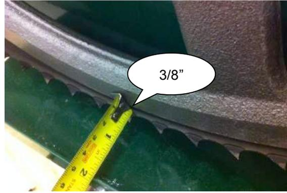
Wearing gloves, spin the bandwheel with your hand and observe how the blade has changed tracking. Measure the distance again and repeat the above step to further compensate if required. The ideal measurement is 3/8" or check for the back of the blade to be flush with the back of the bandwheel.
