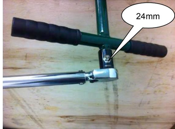
Add waterproof grease to the threads of the blade tension "T" handle and to the washer face that it meets before use. Proper blade tension is achieved when a 24mm socket is used on a torque wrench to tighten the "T" handle to 35 ft-lbs torque. See above right image.
