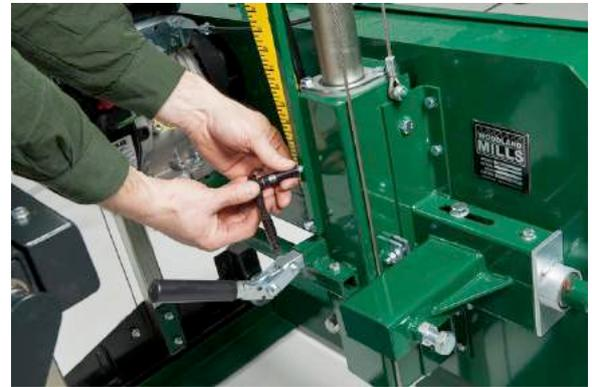
Install the square indicator rod to the sawmill using the two bolts and tighten using a 10mm socket.
