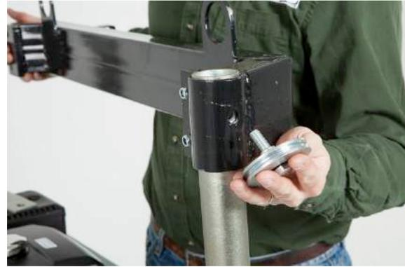
Slide the top cross support over the round post and insert the pulley, collar and bolt assembly into the hole.
