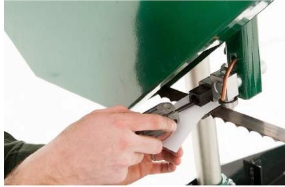
Using a piece of paper in between the blade and blade guide blocks, tighten the allen key bolts.
