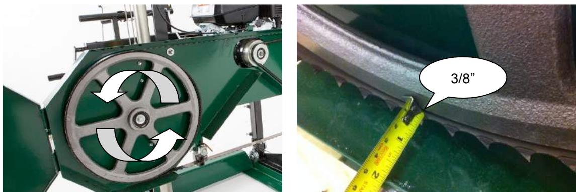
Re-tension the blade by turning the “T” handle a full turn in the clockwise direction. Wearing gloves, spin the bandwheel with your hand and observe how the blade has changed tracking. Measure the distance again and repeat the above step to further compensate if required. The ideal measurement is 3/8” or check for the back of the blade to be flush with the back of the bandwheel.
