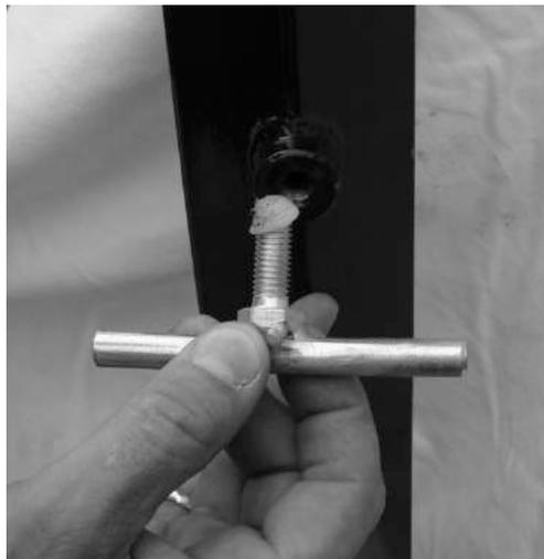
Add grease to all "T" handle threads on the sawmill.
