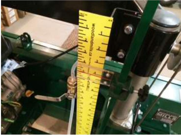
Install the lube tank line to the bracket on the scale by using a Phillips head screw driver and adjustable wrench.
