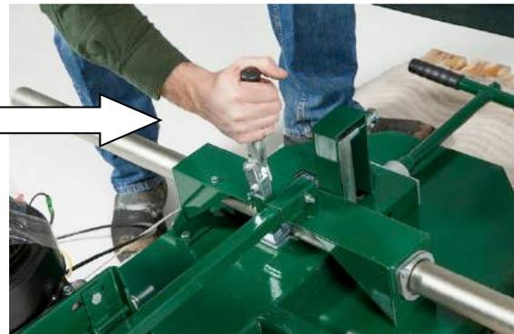
Lock the cam handles on both the round and square post to prevent the head from moving when it is stood up in the coming steps. Ensure that when activating the cam handles, the clamps securely lock on the round and square vertical post. If they don't, a 13mm wrench will need to be used to tighten the adjustment nut. This will allow the clamps to lock on the post better.
