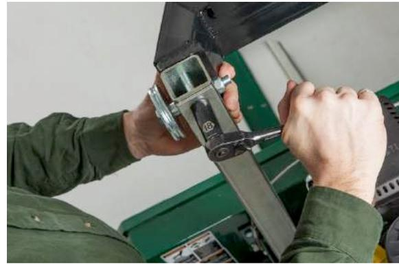
Insert the bolts into the back plate as shown in above left image. Align the square post holes with the corresponding black top cross support holes. Tighten using an 18mm socket.
