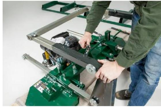
Insert the rear square frame into the carriage base until it bottoms out on the pulley bolts. Tighten the four 16mm bolts (shown in right image) to secure it in place.
