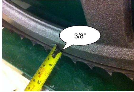
Wearing gloves, spin the bandwheel with your hand and observe how the blade has changed tracking. Measure the distance again and repeat the above step to further compensate if required. The ideal measurement is 3/8".
