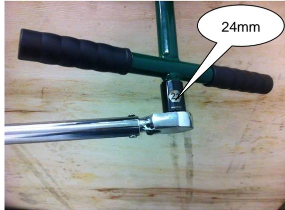
Add grease to the threads of the blade tension “T” handle and to the washer face that it meets before use. Proper blade tension is achieved with a 24mm socket on a torque wrench and is used to tighten the “T” handle to 30-35 ft-lbs torque. See above right image.
