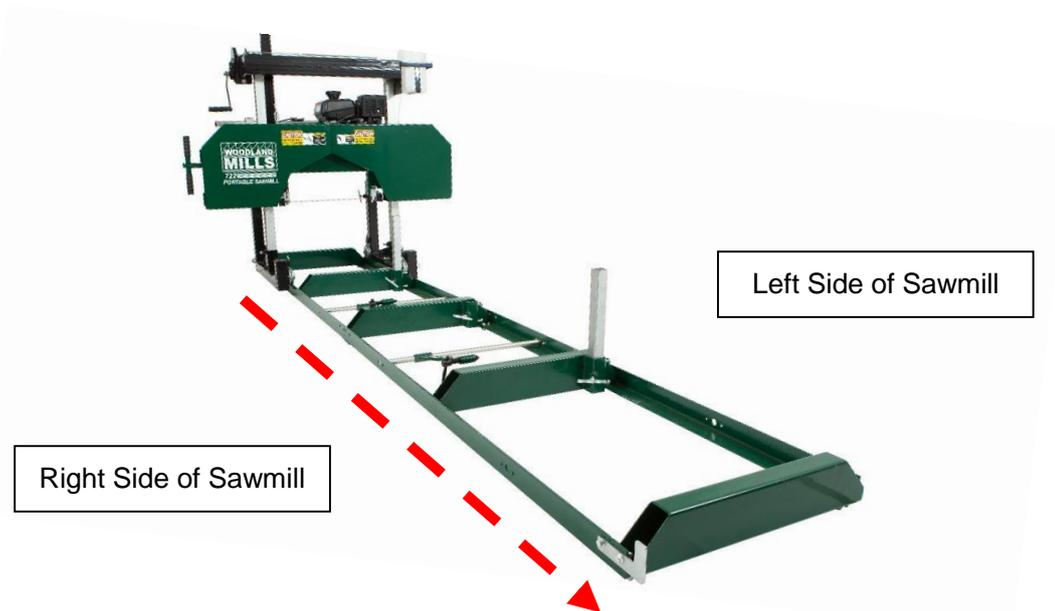
Always cut in the direction shown above. The log clamp should always be on the right side of the log and the log supports should always be on the left. Failure to cut in this direction can cause the log to come loose and possibly even cause damage or injury.
