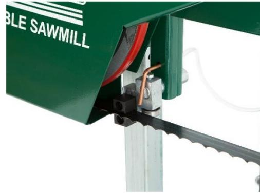
Using the bolts and nuts provided, attach the water valve to the square bar. The end of the hose can be attached to the copper pipe at the blade guide location. Insert the lube tank line through the hole in the bottom of the saw head as shown in above right image. Use a 16mm socket to secure the copper end in position. Do not over tighten or crush the copper end.
