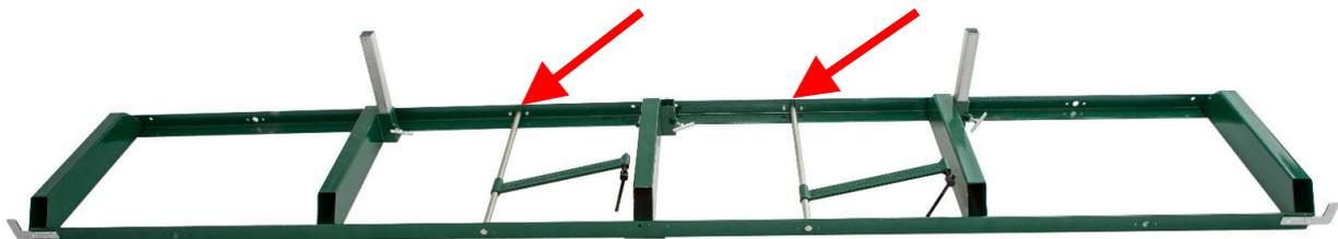
Attach log dog assembly to track as shown above. The rods are secured in place using the 4 nuts and bolts provided. Note that there are various locations along the track where this assembly can be bolted. Depending on how many track sections are being used, select a log clamp position that will secure the log firmly against the log supports.
