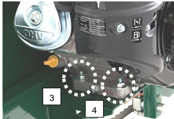
To tighten the drive belt, start by loosening the four bolts that secure the engine to the engine mount.
