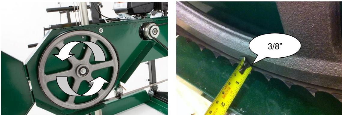
Re-tension the blade by turning the “T” handle a full turn in the clockwise direction. Wearing gloves, spin the bandwheel with your hand and observe how the blade has changed tracking. Measure the distance again and repeat the above step to further compensate if required. The ideal measurement is 3/8”.
