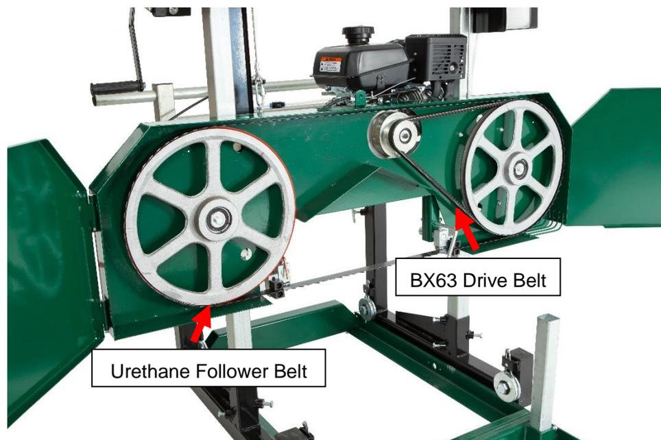
There are two rubber “V” belts on the sawmill and they should be replaced as a set. It is not advised to replace individual belts separately. It is recommended to use a BX63 cogged belt for the drive side and a urethane follower belt.
