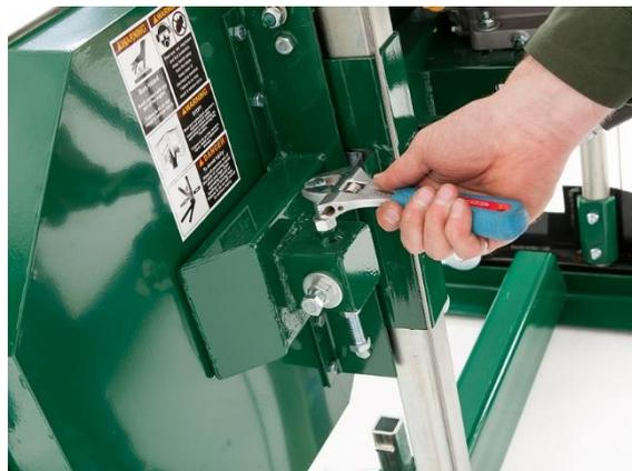
To adjust the left side of the sawmill, again start by taking the tension off of the blade by turning the "T" handle one turn in the counter-clockwise direction. Using a 16mm wrench, loosen the "**vertical nut**" a 1/2 turn. Do the same on the "**bottom vertical nut**". Next, loosen both "**vertical bolts**" a 1/2 turn. This will take the clamping force off of the bandwheel shaft caused by these two bolts and allow it to move freely in the following steps.
