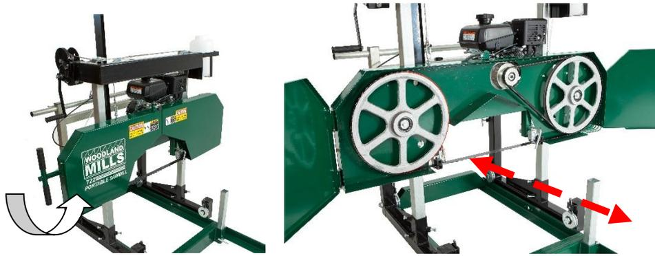
Remove the tension in the blade by turning the “T” handle in the counter-clockwise direction and then open the blade guard cover. The blade should now be loose and free to pull straight out the front.
