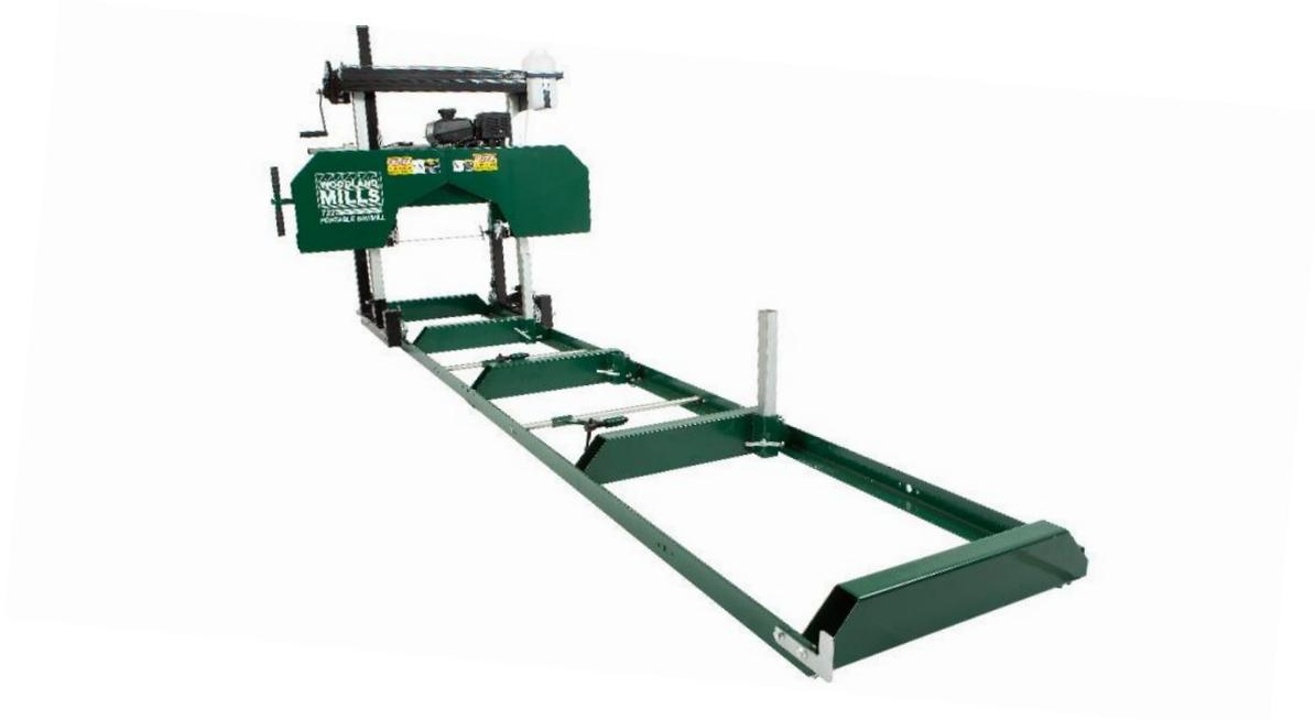
At this point, the saw head should be fully assembled, but not rigidly bolted together. The head can now be set on the tracks as shown above. The following steps will square the head and also firm it up.
