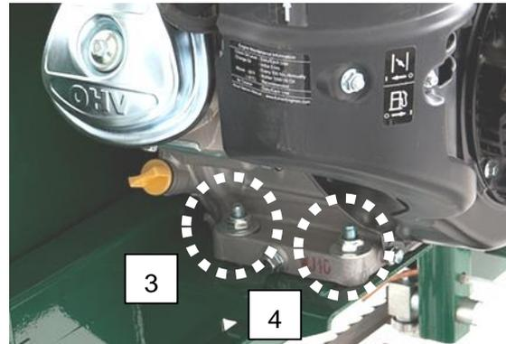
To change the drive side belt, loosen the four bolts that secure the engine to the engine mount using a 16mm wrench.
