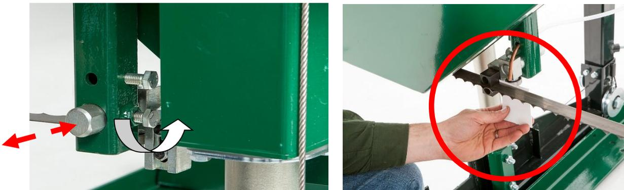
Loosen the blade guide assembly bolt with a 16mm socket. The round shaft should now be free to slide back and forth. Position it so that there is a paper width gap between the bearing and the back of blade. Tighten bolt against the flat on the shaft to secure assembly back in position.
