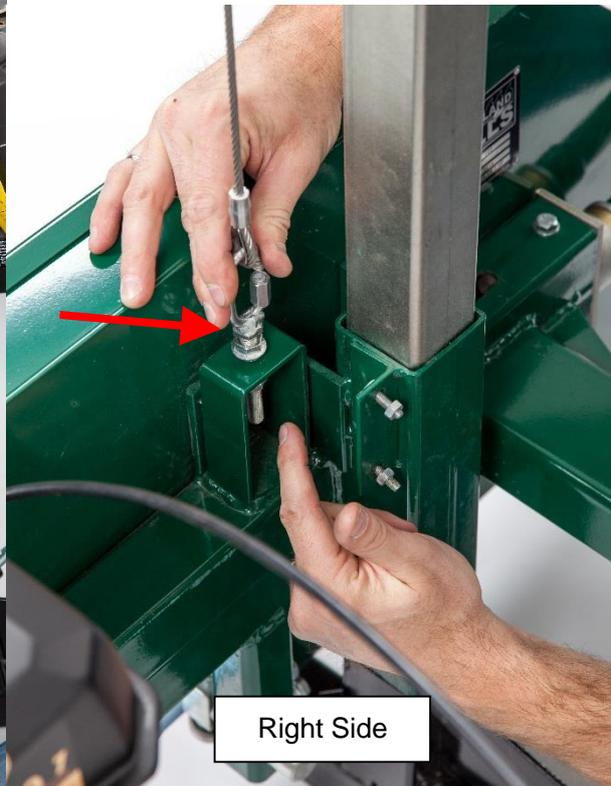
Attach cable ends to head on both sides as shown above. These are adjustable so that the blade/head assembly can be leveled to the log bunks. This will be shown and done at a later step.
