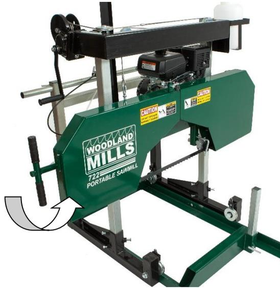
Take some tension off of the blade by turning the “T” handle in the counter-clockwise direction one full turn from full tension position.
