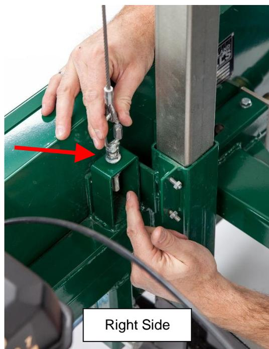
To adjust the head/blade to be level to the cutting deck, the above threaded bolt can be adjusted. The right side of the mill can be lowered by unthreading the bottom nut. To raise the right side of the saw head, the bottom nut can be threaded (up). Once the head is level, the top nut can be tightened to secure the adjuster in place.
