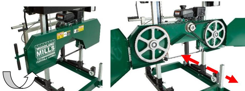
Remove the tension in the blade by turning the “T” handle in the counter-clockwise direction and then open the blade guard cover. The blade should now be loose and free to pull straight out the front. The new blade can now be installed, guards closed and proper blade tension set.
