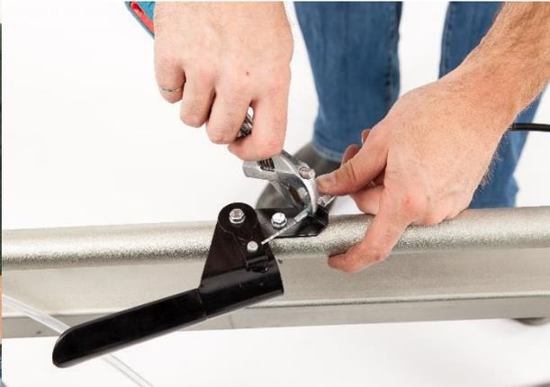
Attach the throttle handle to the rear round bar as shown in the above two images.
