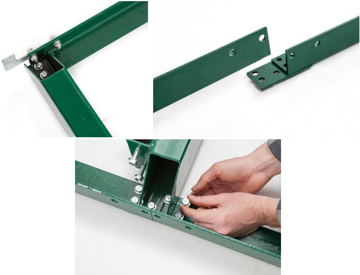
Attach track cross supports to “L” channel with the provided nuts & bolts. The joining plate is used at the seam joint to join the two sections together (shown in top right image). Ensure to only hand tighten at this stage. The bolts will be fully tightened once the head assembly is free to roll on the tracks and provide the correct track width.
