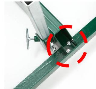
Push the saw head up and down the track system to ensure that the width of the track allows for the saw head to move freely. If it binds, the “L” rails will need to be set further or closer together to achieve a consistent width along the entire track system. Once the desired width is achieved, all nuts and bolts can be tightened to the log bunks as shown in above right image using a 14mm socket.
