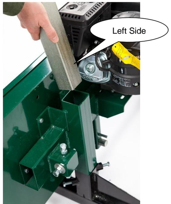
While one person is holding the head in place, have the other person insert both square posts through the head and into the carriage base on both sides. Note that the square post with the two
