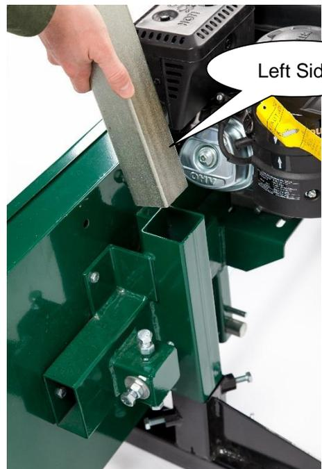
While one person is holding the head in place, have the other person insert both square posts through the head and into the carriage base on both sides. Note that the square post with the two
