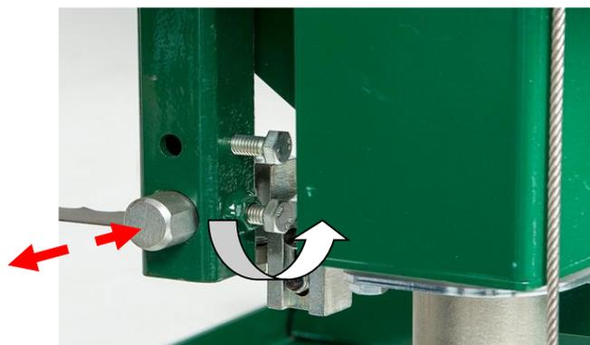
Loosen the blade guide assembly bolt with a 16mm socket. The round shaft should now be free to slide rearward and out of the way. Perform this step on both guide assemblies. This will ensure that the guide bearings do not influence tracking of the blade while adjusting.
