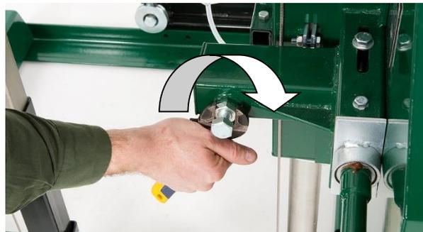
Once satisfied with the measurement, tighten the locking nut clockwise.
