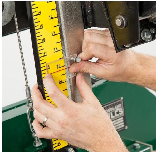
Attach the metal scale bracket to the sawmill head using the two nuts and bolts provided. Use a 10mm socket to tighten. Attach the scale indicator to the post with the two bolts provided and tighten with a 10mm socket. The magnetic log scale can also be placed on the bracket.
