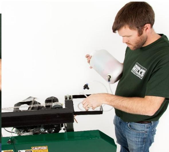
Attach lubrication tank bracket to the left side of the sawmill cross support using the two bolts provided and tighten with a 10mm socket. The lube tank and hose can also be rested into the bracket.
