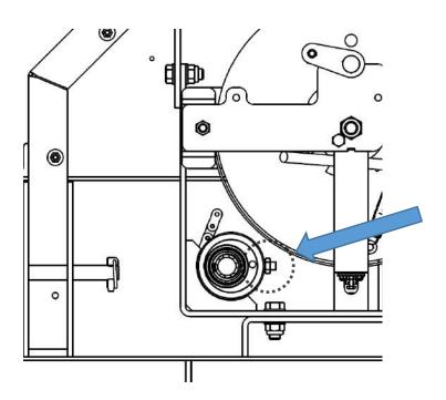
2. Rotate eccentric wheel until desired chain tension is reached.
