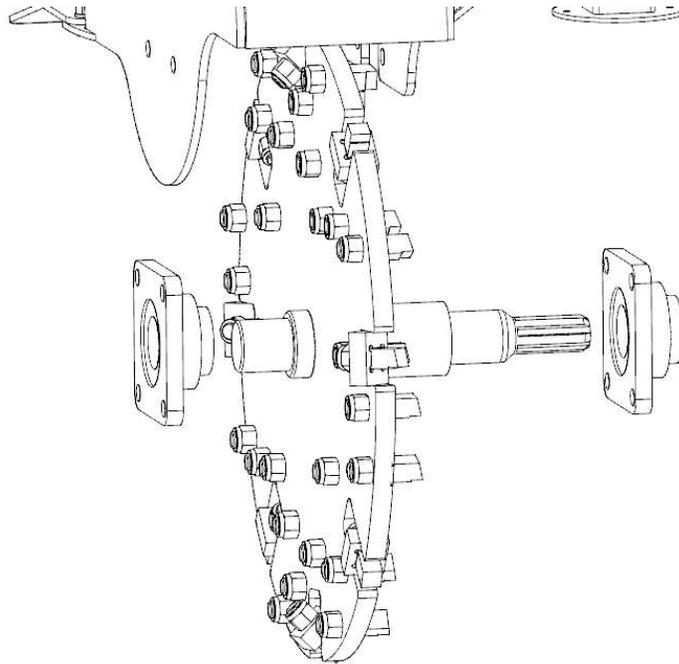
4. Installation is the reverse of removal. Tighten the lock nuts to 65 ft-lbs (88 Nm).
