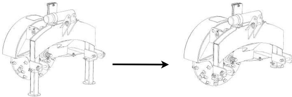
5. Back over a stump and lower the stump grinder so it will take 1" to 4" (25-100mm) per pass. Always make sure the grinder is cutting properly and not jumping around erratically.
