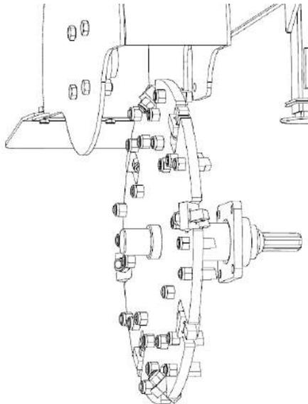
3. Remove the lock nuts and bolts from the remaining bearing and slide the front bearing forward off the flywheel shaft.
