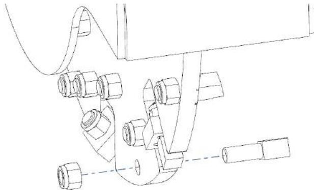
4. Install a replacement tooth and lock nut using a torque wrench set to 160 ft-lbs (215 Nm)
