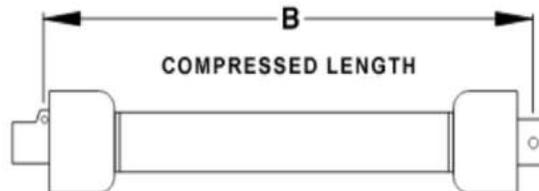
5. If (**A**) is at least 1" longer than (**B**), the PTO shaft will not need to be cut. It is recommended that (**B**) not be used at a dimension any longer than 38".
