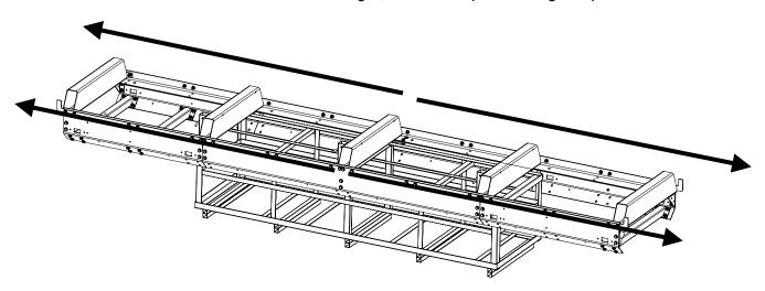
Place the 4 jacks under the end cross beam and the front cross beam and extend the jacks all the way.
