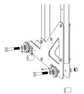
Using the provided M6 x 25 and M6 x 40 bolts, install the brackets in place of the spacers.
