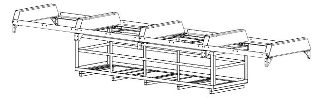
Using the hardware listed below, hang the side plates using the M10x25mm and M10x30mm bolts, do not tighten these bolts. The M10x30mm bolts are used with the track end stop. Everywhere else uses the M10x25mm bolts.
