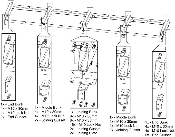
Above steps to be completed to both sides of the track. Make sure the gussets are flush to the outside of the track rails as shown below.
