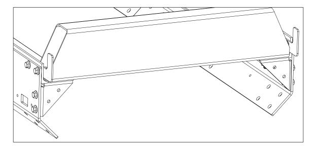
The end stops attach on the inside of the track using the M10 x 30mm bolts.
