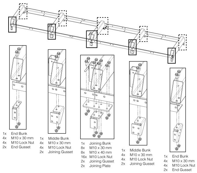
The above steps need to be completed on both left and right sides of the track. Make sure the gussets are flush with the outside face of the track rails as shown below.
