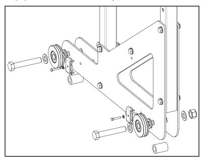
Using the provided M6 X 40 and M6 X 25 mm bolts, install the brackets in place of the spacers. Reuse the four (4) M6 flat washers from the wheel sweepers on the sawmill when replacing the bolts.
