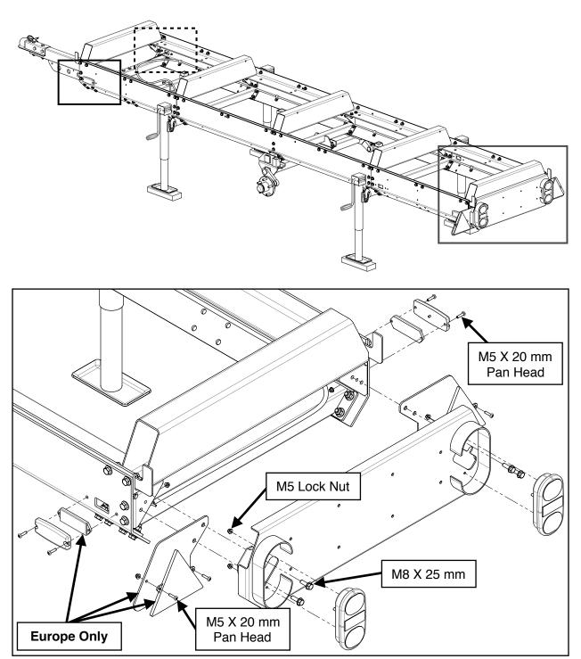
Note: tail lights (North America and Europe) and side lights (North America only) are integral to the wire harness. They are shown exploded for assembly clarity.
