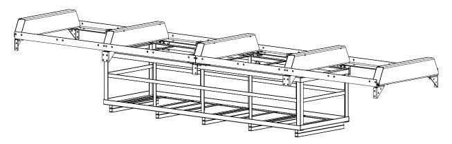
Using the hardware listed below, hang the side plates using the M10 X 30 mm and M10 X 35 mm bolts. Do not tighten these bolts. The M10 X 35 mm bolts are used with the carriage stops. The M10 X 30 mm bolts are used everywhere else.
