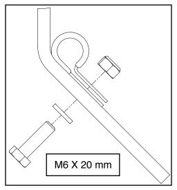
There are 2 cable clamps per short side plate (2) and 4 per long side plate (1) for a total of 8. Cable clamps are installed down the right-hand side of the trailer only. Use the M6 X 20 mm hex bolts, M6 washers, and M6 lock nuts as shown. This applies to both North American and European models.
