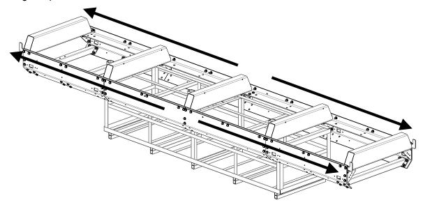
Position the 4 jack stands under the front and rear cross beams and wind the jack handles until they are fully extended.
