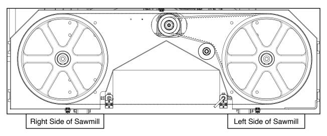
The blade should run with the same tooth to band wheel face distance on both sides:  $\frac{3}{8}$ " (9 mm) is ideal. The back of the blade will be just proud of the back of the band wheel at this distance and is a quicker check than using a tape measure. If an adjustment on either side is required, the below steps detail this procedure.
