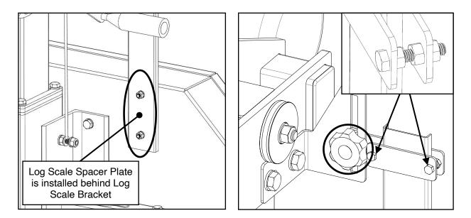
With the hardware listed below, assemble the log scale components.
