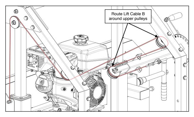
Be sure to securely tighten the oval chain link with a wrench after the cable loop ends have been attached.
