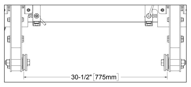
To adjust the width of the wheels, washers may be added or removed from each wheel to ensure a distance of 30-1/2" (775 mm) is achieved as shown below.
