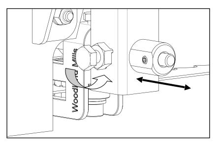
Take some tension off the blade by turning the T-handle in the counter-clockwise direction one full turn from its fully-tensioned position.
