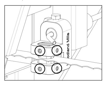
Loosen the blade guide assembly bolt using a socket/wrench. The round shaft should now be free to slide back and forth. Position it so that there is a thick paper-sized gap (.040" or 1 mm) between the bearing and the back of blade. Tighten the bolt against the flat on the shaft to secure the assembly back into position.
