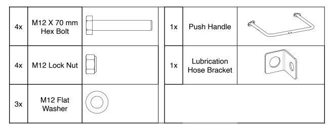
Attach the push handle to the side of the post using four (4) M12 X 70 mm bolts, three (3) M12 washers, and four (4) M12 lock nuts as shown below. Be sure to attach the nut to the water line bracket without a washer. Fully tighten these bolts.
