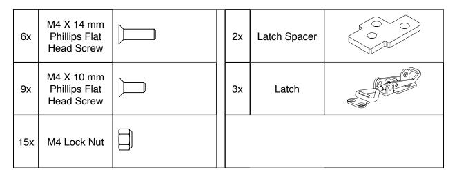
Using a Phillips head screwdriver and a socket/wrench, install the upper latch using five (5) M4 X 10 mm Phillips flat head screws and M4 lock nuts. Install each of the bottom latches with a spacer, three (3) M4 X 14 mm Phillips flat head screws, two (2) M4 X 10 mm Phillips flat head screws, and five (5) M4 lock nuts. The longer screws pass through the three (3) holes in each of the spacers.
