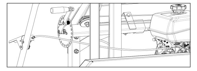
The assembled throttle handle and routed cable should now match the image below.
