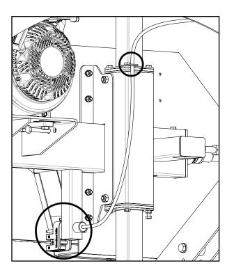
Insert the lubrication hose as shown below. Use a hex wrench to secure the copper end in position by tightening the set screw so that it lightly pinches the copper tube. Do not over-tighten or the end of the copper tube could be crushed.
