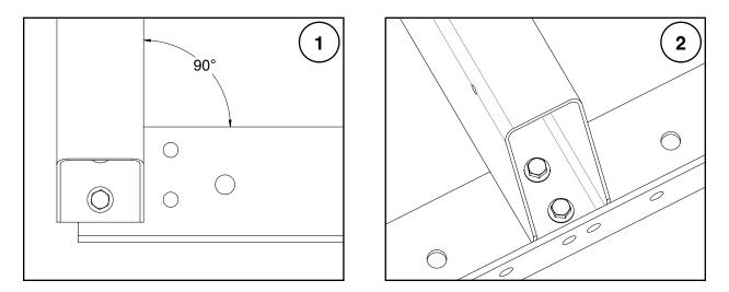
Use sixteen (16) M10 X 35 mm bolts to join the centre bunk and reinforcement plates to the rails at the rail joints (Figure 3).
