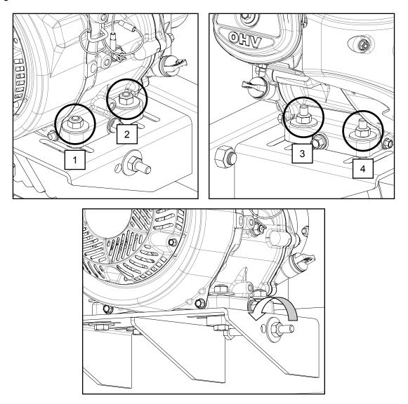
Now that the engine is free to slide on the engine mounting plate, turn the nut on the horizontal stud in the counter-clockwise direction. This will allow the engine to move and also take the tension off of the belt. The old belt can now be removed and the new belt installed. Tension the new belt and refer to the <u>BELT TENSION</u> instructions described in the <u>SAWMILL SET-UP</u> <u>PROCEDURES</u> section of the manual.
