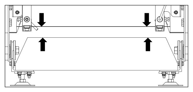
Using a wrench, turn the nut clockwise to raise one side of the sawmill head assembly, or counter-clockwise to lower it. Double-check the blade height as discussed in the previous step. Once the measurements are equal on both sides, tighten the corresponding jam nut to clamp it securely against tab.
