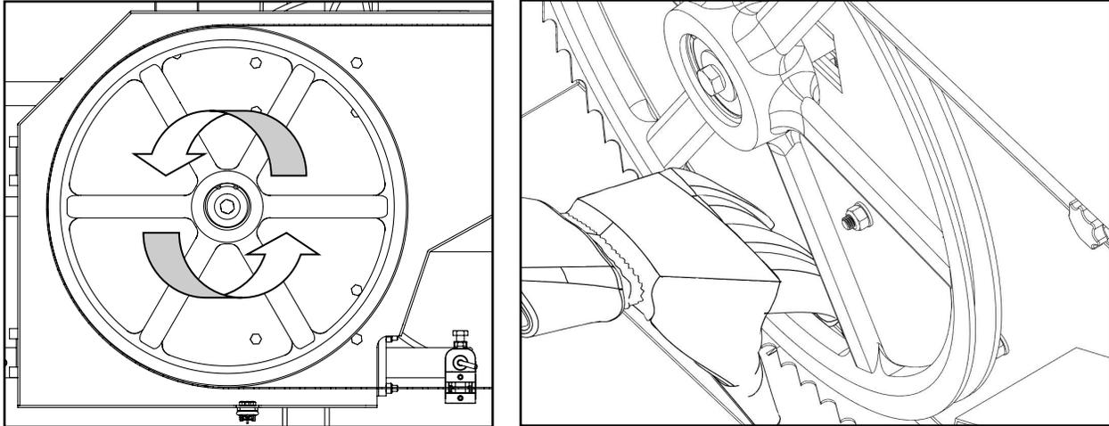
Once satisfied with the measurement, tighten the locking nut clockwise.
