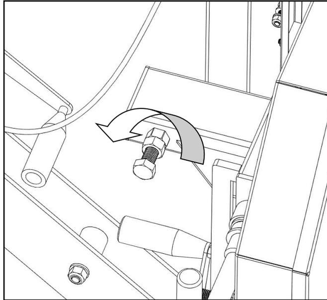
The alignment bolt can now be turned to change the angle of the band wheel and track the blade. To move the blade more rearward on the band wheel, turn this bolt clockwise. Alternatively, turning the bolt in the counter-clockwise direction will force the blade to run more forward on the band wheel. Turn the bolt ½ turn and re-tension the blade.
