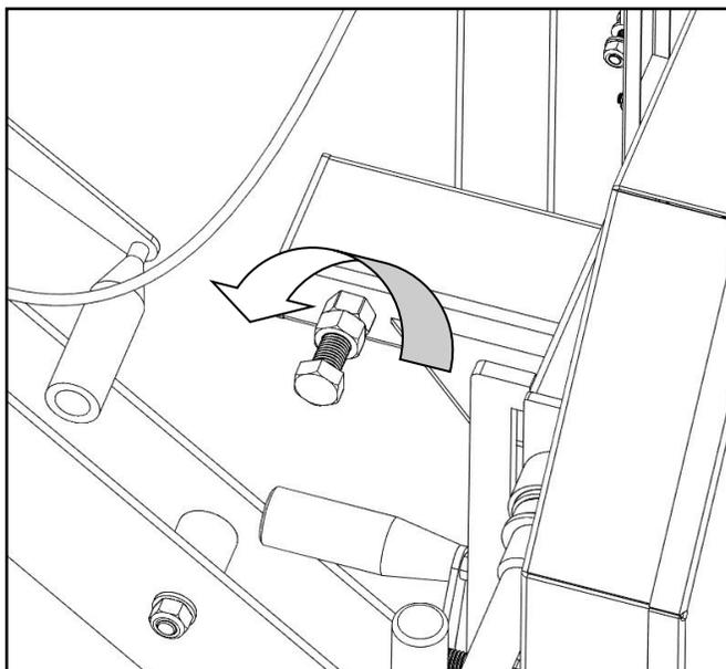
The alignment bolt can now be turned to change the angle of the band wheel and track the blade. To move the blade more rearward on the band wheel, turn this bolt clockwise. Alternatively, turning the bolt in the counter-clockwise direction will force the blade to run more forward on the band wheel. Turn the bolt  $\frac{1}{2}$  turn and re-tension the blade.
