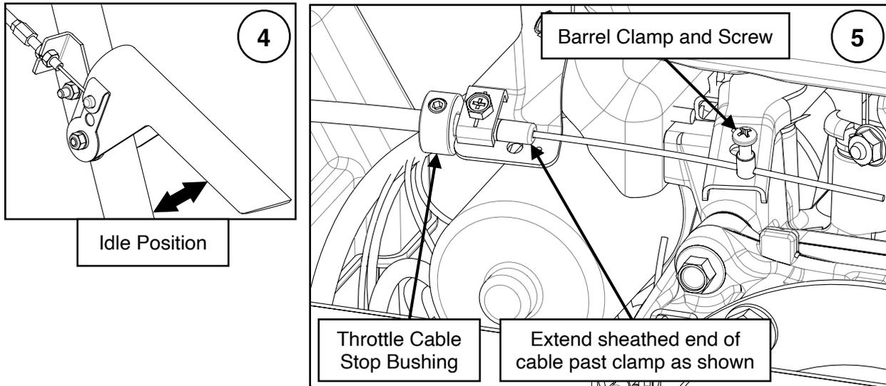
Finally, slide the throttle cable stop bushing along the cable sheath until it stops at the bracket on the engine. Secure it in place by tightening the set screw with a 3 mm hex key.
