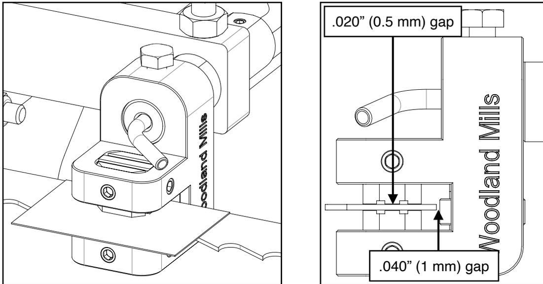
After the guide blocks and guide rollers are set, slide the adjustable blade guide in and out while noting the blade guide bearing-to-blade gap and the guide block-to-blade gap. If either of these gaps change while sliding the guide block adjustment arm, the guide angle can be adjusted via the steps on the next page.
