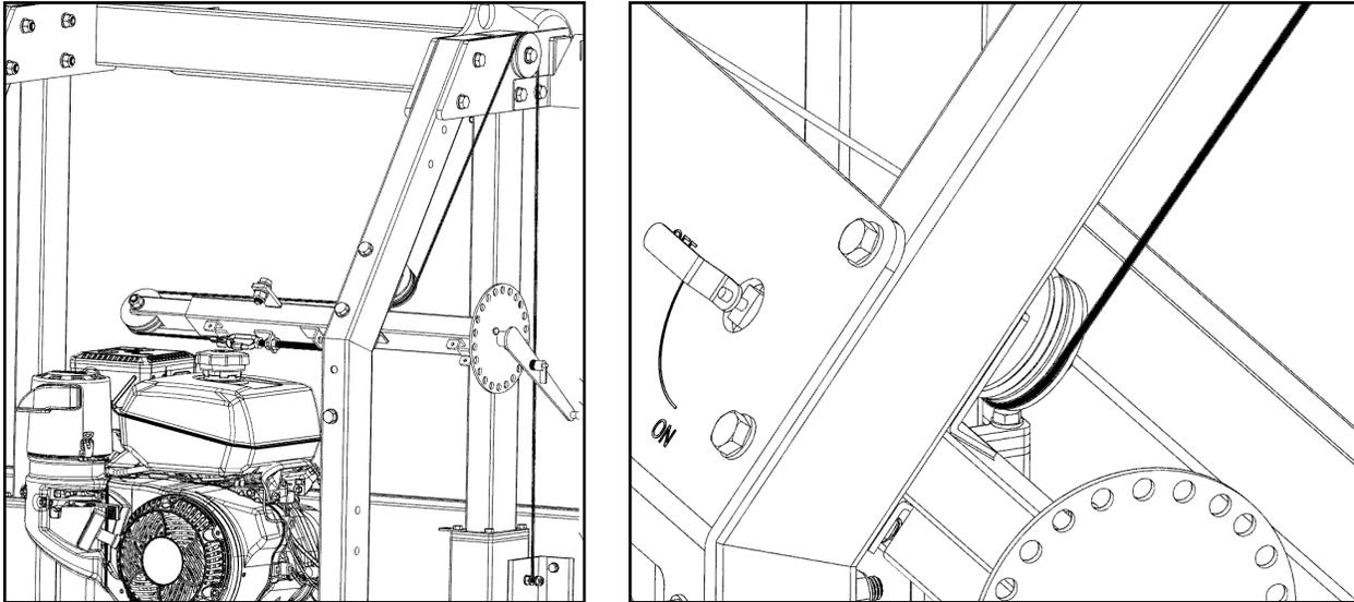
Be sure to securely tighten the oval chain link with a wrench after the cable loop ends have been attached.
