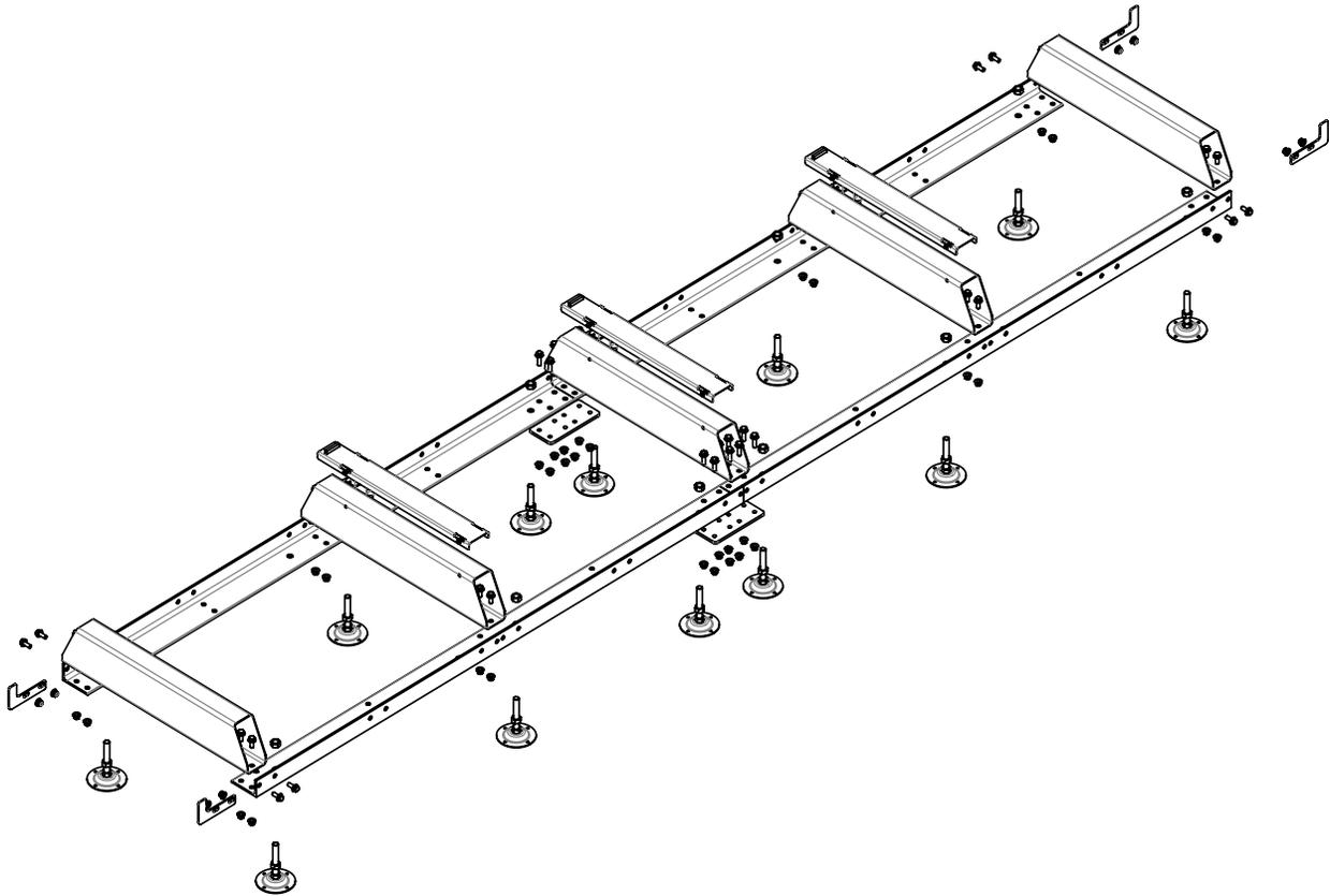
When assembling the log bunks to the rails, ensure that the two end bunks are square ( $90^\circ$ ) as shown in Figure 1. Note that the two (2) end bunks will not have stainless steel bunk caps attached. Use sixteen (16) M10 X 25 mm bolts at all end bunk and mid bunk locations (Figures 1 & 2).
