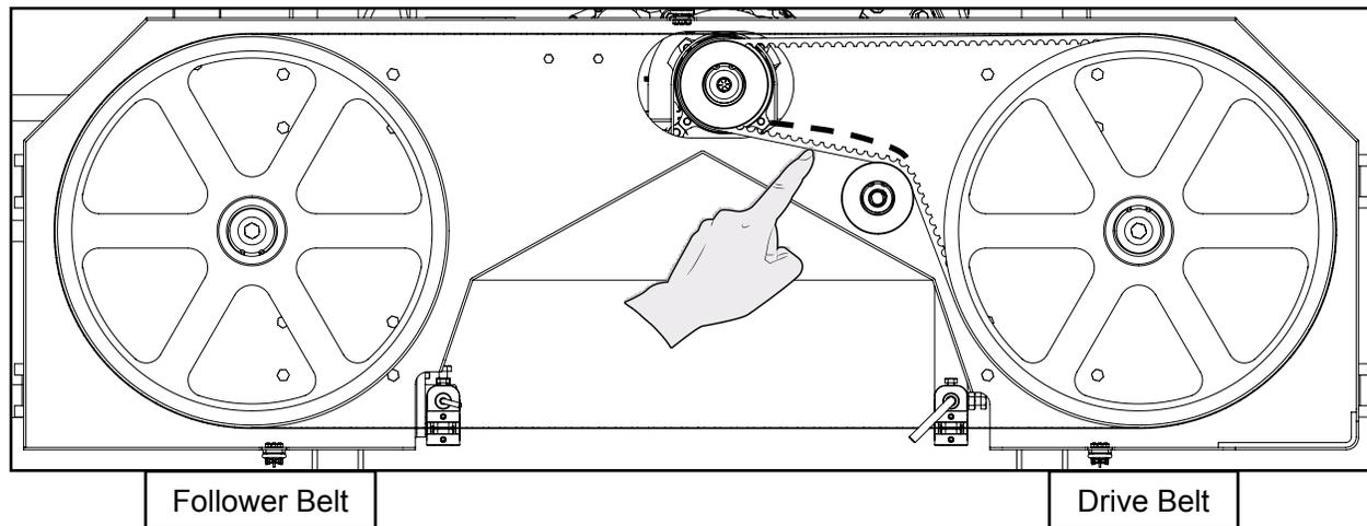
**\*\*Never attempt to adjust the belt tension with the engine running. As a safety precaution, remove the spark plug cap.\*\***
