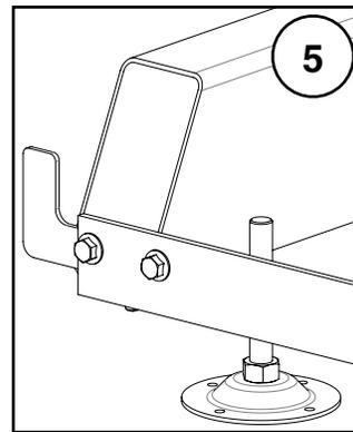
Assemble the four (4) carriage stops to the ends of the rails and tighten the bolts. Ensure carriage stops are assembled to the inside face of the rails, *not* the outside (Figure 5).
