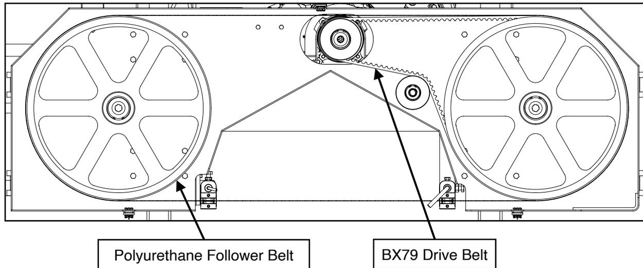
Remove the tension in the blade by turning the T-handle in the counter-clockwise direction and then open the blade guard cover. The blade should now be loose and free to pull straight out the front.
