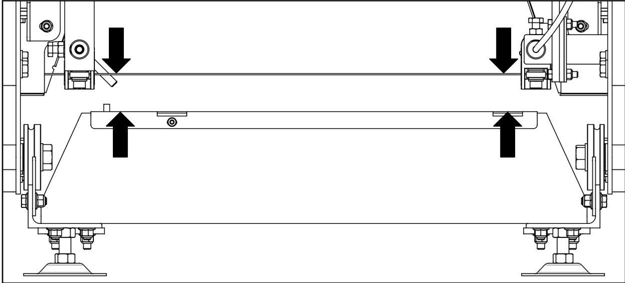
Using a wrench, turn the nut clockwise to raise one side of the sawmill head assembly, or counter-clockwise to lower it. Double-check the blade height as discussed in the previous step. Once the measurements are equal on both sides, tighten the corresponding jam nut to clamp it securely against tab.
