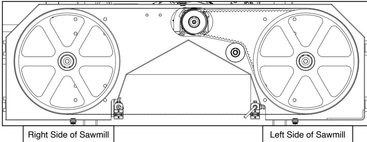
The blade should run with the same tooth to band wheel face distance on both sides:  $\frac{3}{8}$ " (9 mm) is ideal. The back of the blade will be just proud of the back of the band wheel at this distance and is a quicker check than using a tape measure. If an adjustment on either side is required, the below steps detail this procedure.
