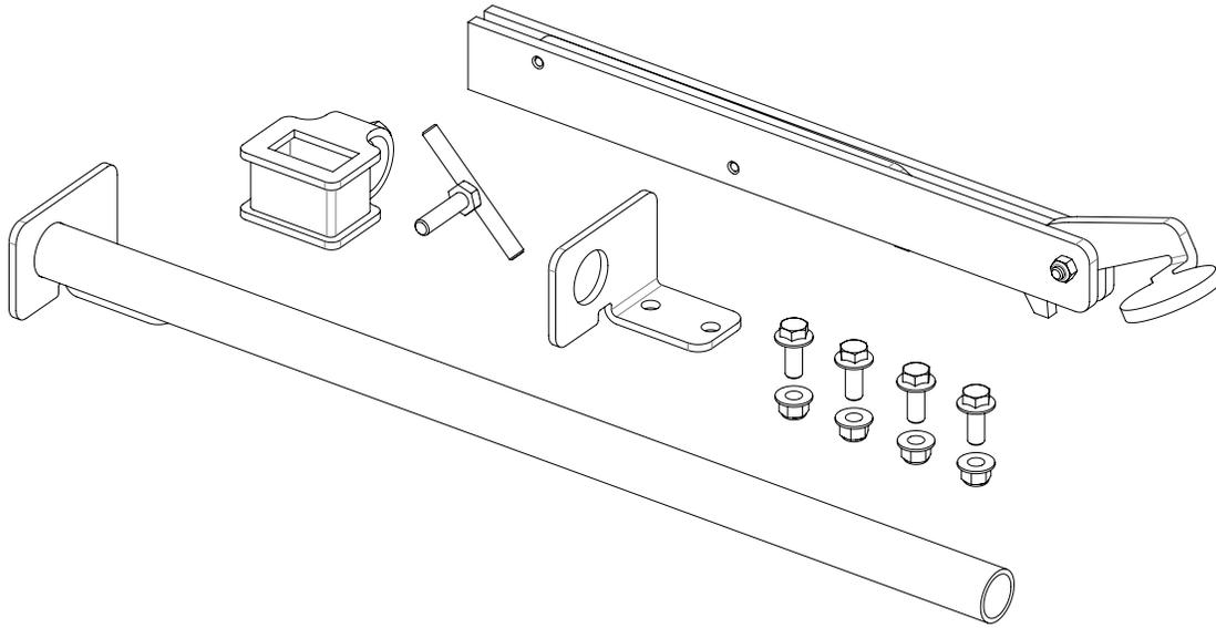
Attach log dog assembly to track as shown below with the four (4) nuts and bolts provided. Note that there are various locations along the track where this assembly can be bolted. Depending on how many track sections are being used, select a log clamp position that will secure the log firmly against the log supports.
