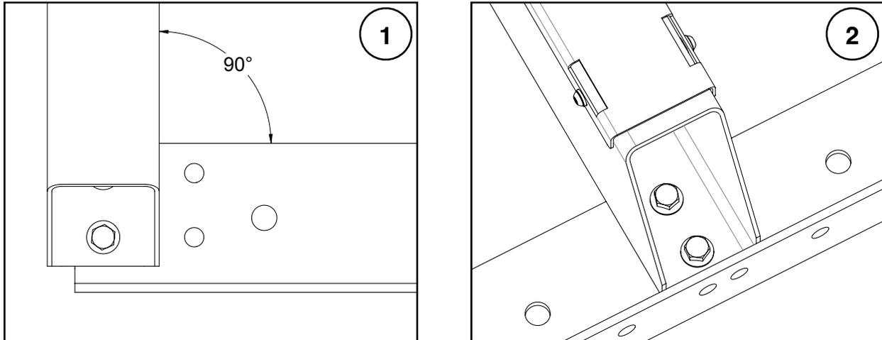
Use sixteen (16) M10 X 35 mm bolts to join the centre bunk and reinforcement plates to the rails at the rail joints (Figure 3).
