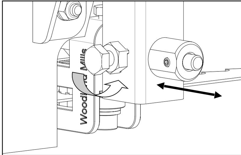
Take some tension off the blade by turning the T-handle in the counter-clockwise direction one full turn from its fully-tensioned position.
