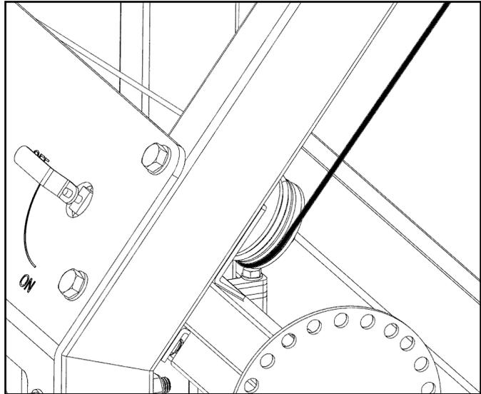
Be sure to securely tighten the oval chain link with a wrench after the cable loop ends have been attached.
