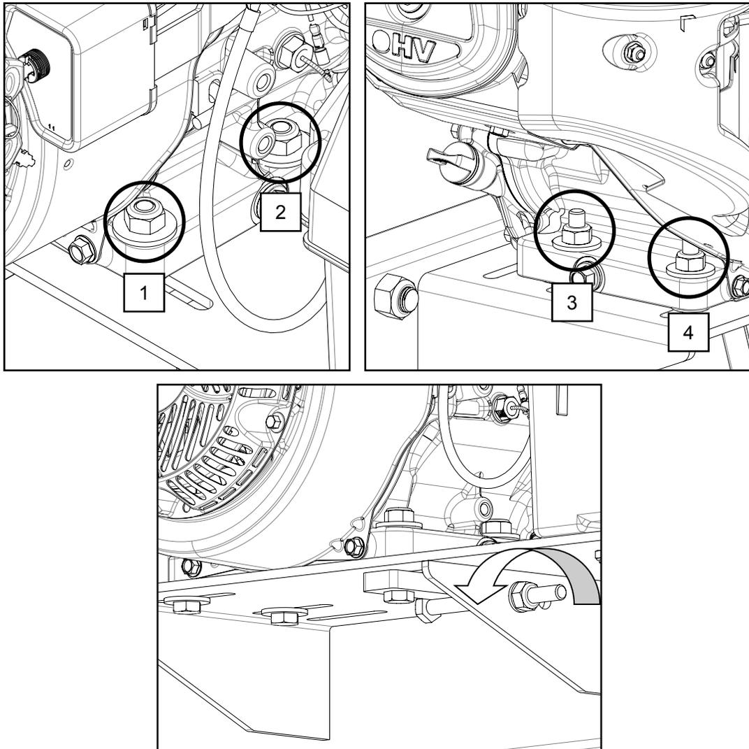
Now that the engine is free to slide on the engine mounting plate, turn the nut on the horizontal stud in the counter-clockwise direction. This will allow the engine to move and also take the tension off of the belt. The old belt can now be removed and the new belt installed. Tension the new belt and refer to the **BELT TENSION** instructions described in the **SAWMILL SET-UP PROCEDURES** section of the manual.
