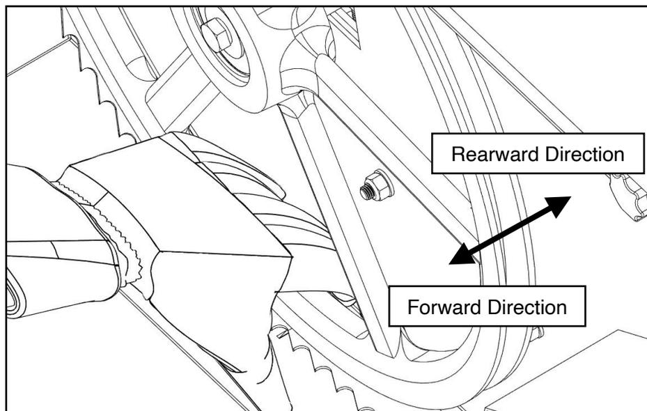
Loosen the blade guide assembly bolt using a socket/wrench. The round shaft should now be free to slide rearward and out of the way. Perform this step on both blade guide assemblies. This ensures the guide bearings will not influence tracking of the blade whilst being adjusted.
