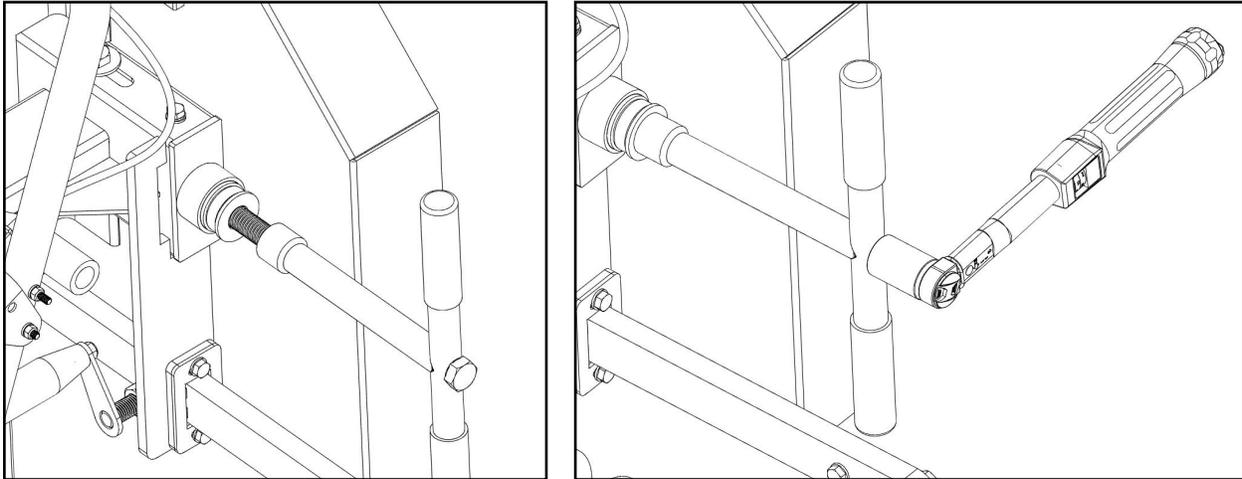
**\*\*Note: It is very important to take the tension off the blade by turning the T-handle in the counter-clockwise direction when the sawmill is not in use. Failure to do so will result in flat spots on the rubber belts. These flat spots will cause the mill to vibrate excessively during next use.\*\***
