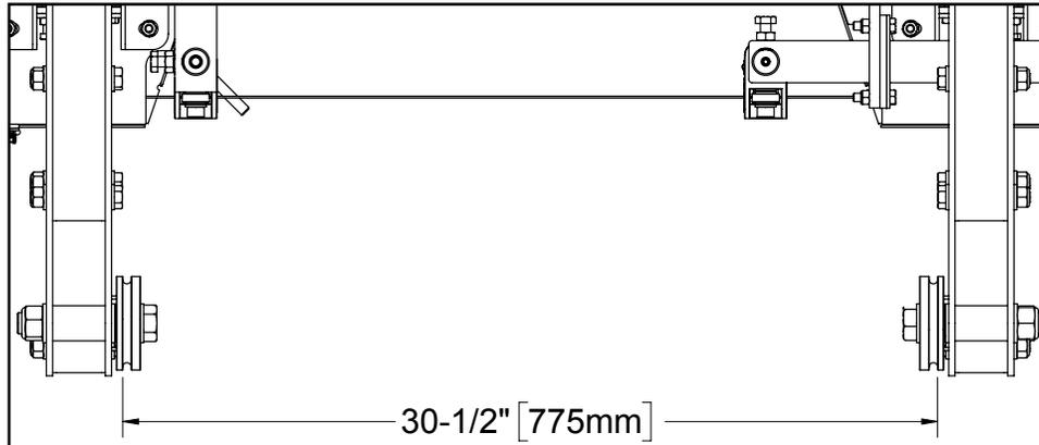
To adjust the width of the wheels, washers may be added or removed from each wheel to ensure a distance of 30.5" (775 mm) is achieved as shown below.
