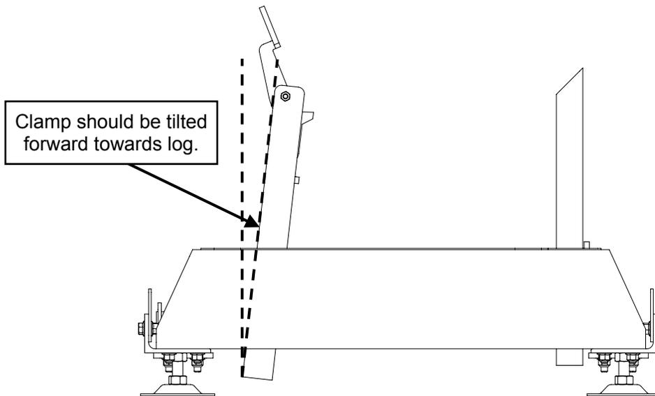
Insert log supports into track cross supports and secure with T-handles as shown in the picture below. The T-handle threads should be coated with grease. The sawmill includes two sets of log supports—a short set and a long set. The long set is ideal for large diameter logs while the shorter set is better suited for small logs and square cants.
