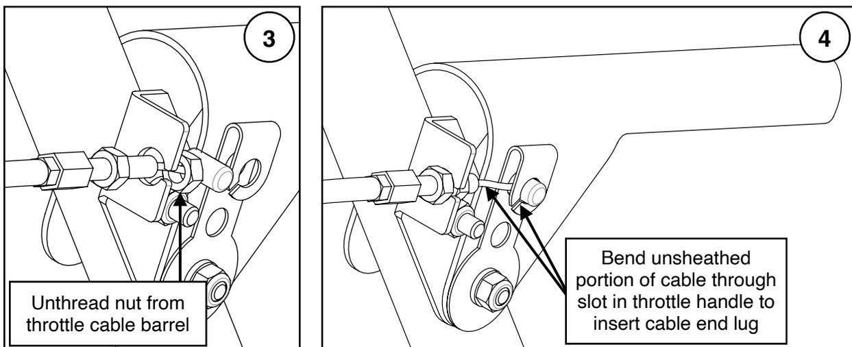
With the throttle lever in the idle position (fully open), slide the *throttle cable stop bushing* over the end of the cable sheath and pull the cable tight at the engine. The sheathed end of the cable should extend past the clamp on the engine (see Figure 2). Next, pass the unsheathed end of the cable through the hole in the barrel clamp and tighten the M4 Phillips pan head screw to secure it in place. This will take the slack out of the cable.
