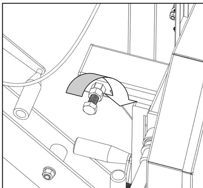
Tighten the blade tension back to 25 ft•lb (34 N•m). While wearing gloves, spin the band wheel with your hand and observe how the blade tracking has changed. Measure the distance again and repeat the above step to further compensate if required. The ideal measurement is  $\frac{3}{8}$ " (9 mm) or check that the back of the blade is flush with the back of the band wheel.
