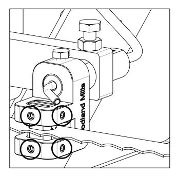
Loosen the blade guide assembly bolt using a socket/wrench. The round shaft should now be free to slide back and forth. Position it so that there is a thick paper-sized gap (.040" or 1 mm) between the bearing and the back of blade. Tighten the bolt against the flat on the shaft to secure the assembly back into position.
