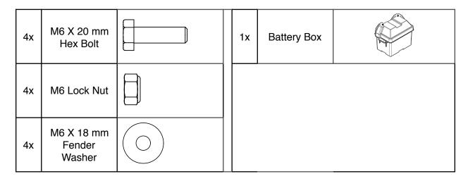
Using two (2) sockets/wrenches, install the battery box with four (4) M6 X 20 mm bolts, M6 fender washers, and M6 lock nuts as shown in the image below.
