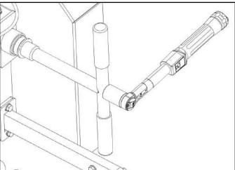
\*\*Note: It is very important to take the tension off the blade by turning the T-handle in the counter-clockwise direction when the sawmill is not in use. Failure to do so will result in flat spots on the rubber belts. These flat spots will cause the mill to vibrate excessively during next use.\*\*
