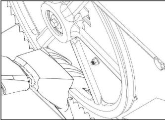
Once satisfied with the measurement, tighten the locking nut clockwise.
