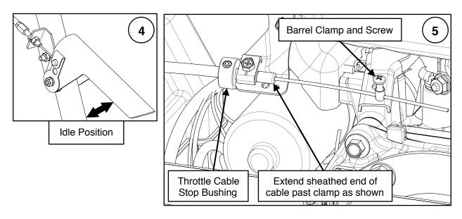
Finally, slide the throttle cable stop bushing along the cable sheath until it stops at the bracket on the engine. Secure it in place by tightening the set screw with a 3 mm hex key.
