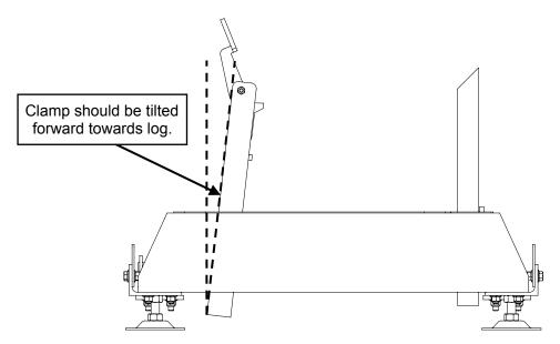
Insert log supports into track cross supports and secure with T-handles as shown in the picture below. The T-handle threads should be <u>coated with grease</u>. The sawmill includes two sets of log supports—a short set and a long set. The long set is ideal for large diameter logs while the shorter set is better suited for small logs and square cants.
