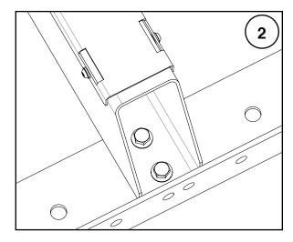
Use sixteen (16) M10 X 35 mm bolts to join the centre bunk and reinforcement plates to the rails at the rail joints (Figure 3).
