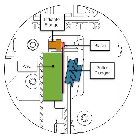
The tooth to be offset must always point toward the indicator plunger. When a tooth is offset over the anvil, the bend starts at the *gullet*. Adjust the two (2) screws shown below to ensure the blade is sitting level and that the tooth will bend over the anvil at the gullet line.
