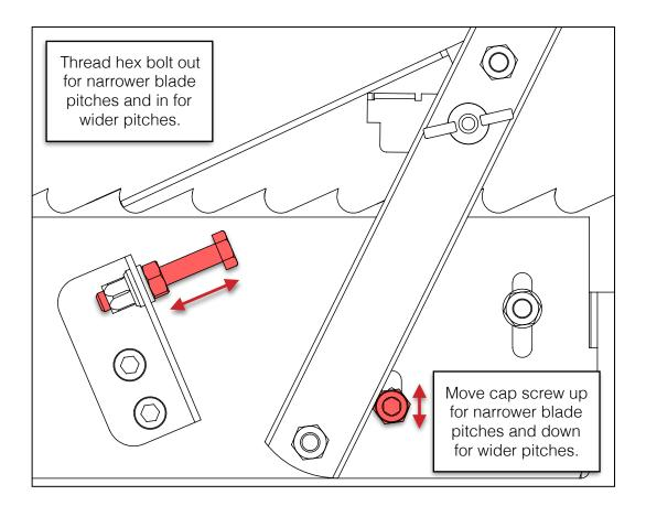
\*\*Depending on the blade pitch, it may take a combination of adjustments from both the hex bolt and the cap screw to set the correct spacing.\*\*
