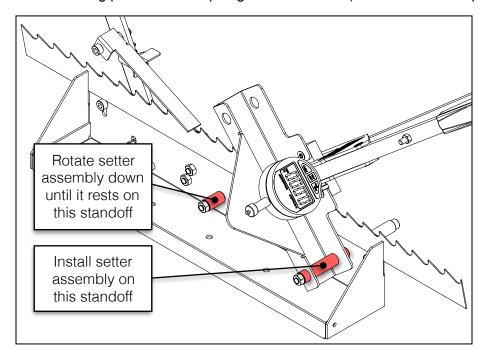
To set the teeth that point in the opposite direction (towards the inside of the blade band), reverse the installation of the setter by mounting it to the rear of the base as shown below.
