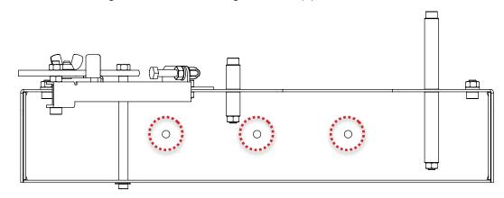
Insert the blade into the slots located at each end of the base as shown.
