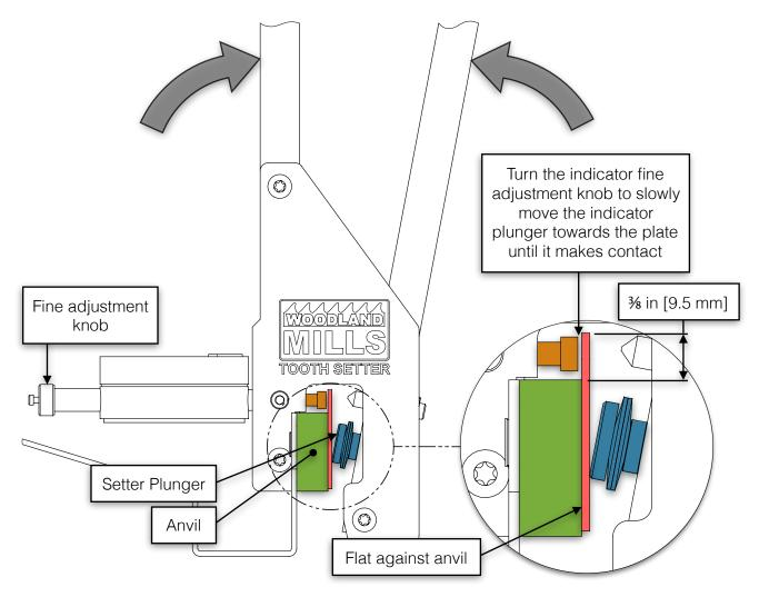
Squeeze the setter handles together with light pressure, just enough to push the calibration plate flat against the anvil.
