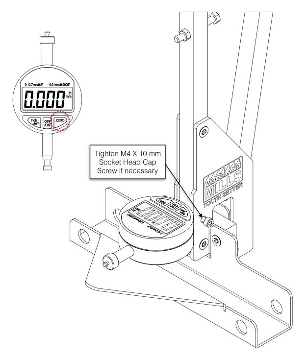
Fully tighten the M4 X 10 mm socket head cap screw using the provided M3 hex key if necessary.
