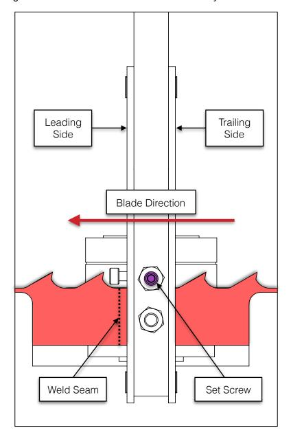
\*\*Always start the setting process with the weld seam on the leading side of the setter head, just past the set screw and indicator plunger.\*\*
