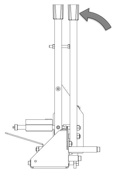
As an initial test to achieve a final tooth offset of .0215 in [0.55 mm], bend it .047 in [1.2 mm] and check the measurement after spring-back. The measurement may vary depending on the thickness of the blade band, initial offset of the tooth before setting, or the blade material itself.
