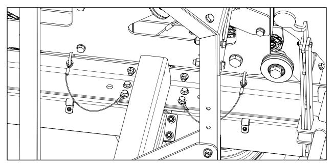
\*\*Remember to continue to use the standard lock-down plates on the left side of the carriage when transporting the sawmill.\*\*
