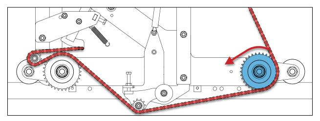
Now route the cable portion of the cable chain under the chain adjustment bracket pulley and hook the open loop end on the extension spring.
