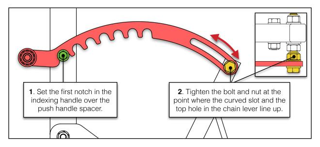
Adjust the middle and end nuts on the indexing handle to better position the handle over the push handle spacer. Fully tighten the hardware once positioned correctly.
