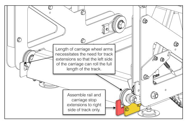
First, remove the existing carriage stops from both ends of the right-side track rails.
