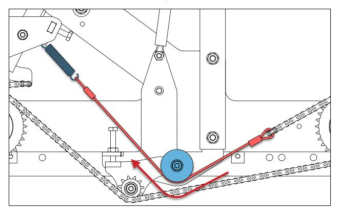
As long as the extension spring is under even a small amount of tension, the cable chain routing is acceptable.
