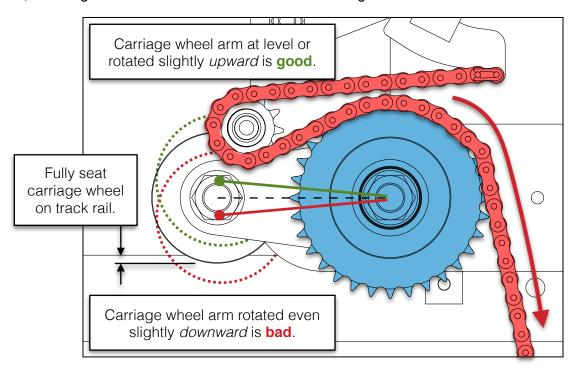
If the arm is rotated even slightly downward, remove the chain from the arm sprocket, rotate the arm until it is level or pointing just slightly upward, and then reset the chain.
