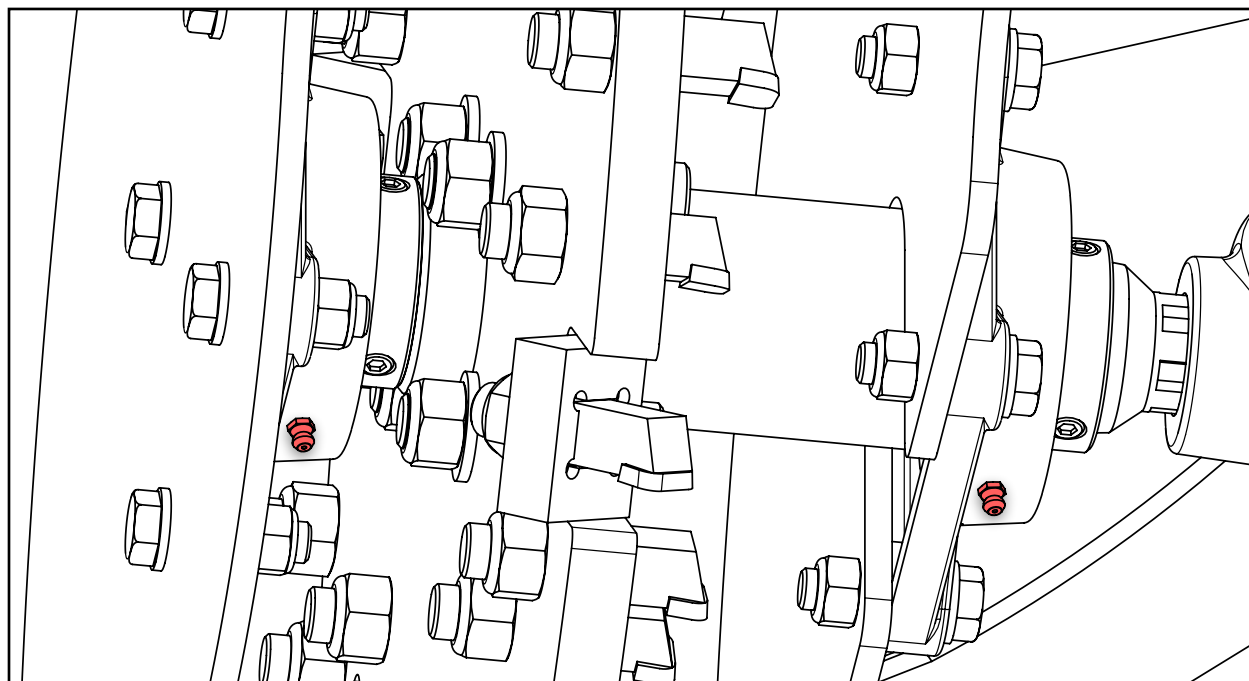
Flywheel Shaft Bearings (Underside of Flywheel Housing)
