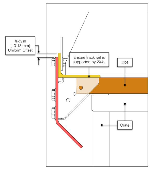
If the offset is not uniform, ensure the track is sitting on the 2X4s and not the crate. The side plates need to hang from the rails unobstructed, with only the force of gravity pulling them down.
