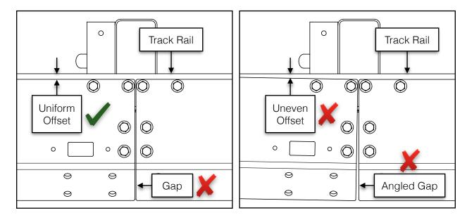
If there are gaps, or if the short side plates are not hanging parallel to the top of the track rails, the included ratchet strap can be used to pull the plates together before torquing the bolts in a similar manner to, **STEP 6. CENTRE BUNKS**, as shown on the next page.
