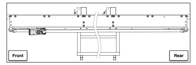
Remember to maintain a uniform offset between the top of the track rails and the top of the side plates when tightening the strap.
