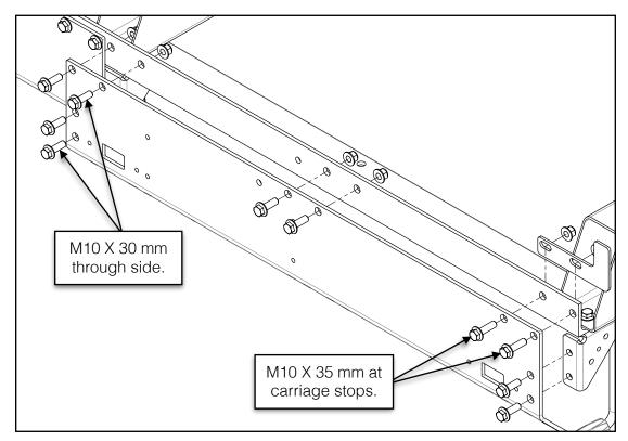
With the long side plates already secured in place, note the gaps (if any) between the short side plates and the long side plates.
