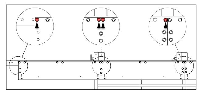
With the front long side plate secured in place, note the gaps (if any) between the rear long side plate and the front long side plate.
