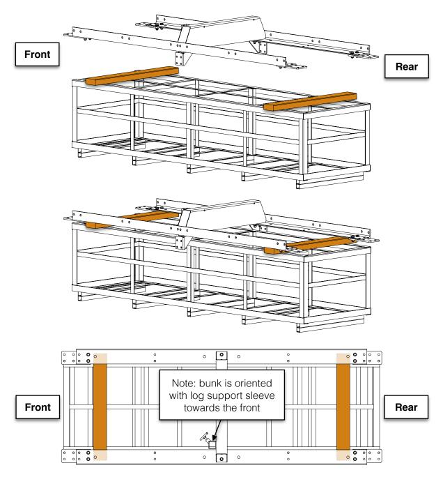
For either the HM126 or HM130, use 30 in [762 mm] long 2X4s. Use 36 in [914 mm] long 2X4s for the HM130MAX.
