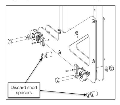
Using the provided M6 X 40 mm and M6 X 25 mm bolts, install the lock-down plates in place of the short spacers with the taller spacer sandwiched between. Reuse the four (4) M6 flat washers from the wheel sweepers on the sawmill when replacing the bolts.
