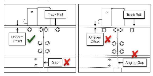
If there are gaps, or if the rear long side plate is not hanging parallel to the top of the track rails, the included ratchet strap can be used to pull the plates together before torquing the bolts as shown on the next page.
