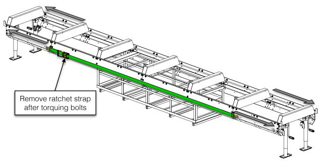
With all of the bolts now tightened, lower the jacks so that the assembly is resting entirely on the crate.
