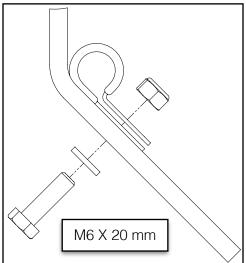
There are 2 cable clamps per short side plate (2) and 4 per long side plate (2) for a total of 12. Cable clamps are installed down the right-hand side of the trailer only. Use the M6 X 20 mm hex bolts, M6 washers, and M6 lock nuts as shown. This applies to both North American and European models.
