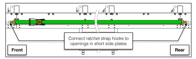
Remember to maintain a uniform offset between the top of the track rails and the top of the side plates when tightening the strap.
