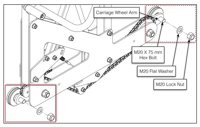
Install the pre-assembled wheel sweeper bracket on the M20 X 75 mm hex bolt using the M20 flat washer and M20 lock nut. Ensure that the rear bracket is properly oriented to avoid the rear idler. Fully tighten the hardware.
