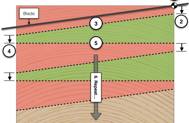
Note: the notches in the indexing handle do not represent fixed angles. The sawhead angle will vary depending on sawmill model.
