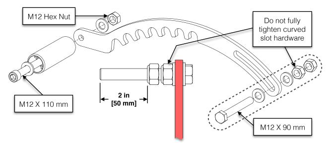
Leave approximately 2 in [50 mm] from the end of the bolt to the first lock nut at the curved slot.
