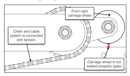
Loosen and undo any adjustment made to the chain adjustment bracket in the previous step. This step requires the assistance of one or more people: lift the *right side* of the sawhead approximately 2 inches up off the setup blocks. Skip one chain link on the front-right carriage wheel arm, moving the carriage wheel arm downward.
