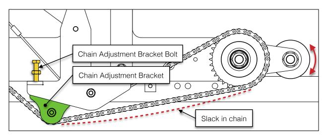
Tighten the chain adjustment bracket bolt by turning it clockwise until the slack is taken up and the carriage wheel binds with the track rail.
