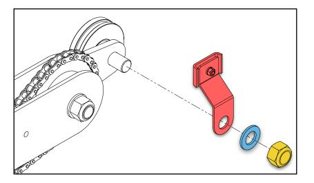
Once the wheel sweeper brackets are both properly positioned, install the wheel sweeper cables. Fully tighten the M6 X 20 mm hex bolts that were installed during the wheel sweeper bracket pre-assembly.
