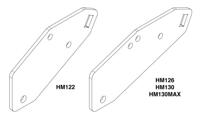
The lever plate for the HM126, HM130, and HM130MAX works with all three (3) sawmill models. Care must be taken to assemble the spacer to the proper hole in the lever plate depending on the model.
