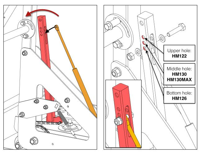
\*\*Assemble the gas spring to the chain lever using the <u>upper</u> lever hole for HM122, the <u>middle</u> hole for HM130 & HM130MAX, and the <u>bottom</u> lever hole for HM126.\*\*
