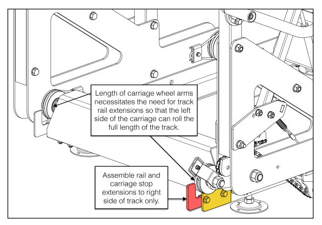
First, remove the existing carriage stops from both ends of the right-side track rails.
