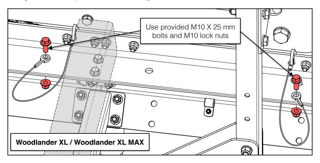
The lanyards prevent the travel hooks from getting lost when the sawmill trailer is not being transported. Be sure to remove the hooks from the top of the rail before milling lumber.
