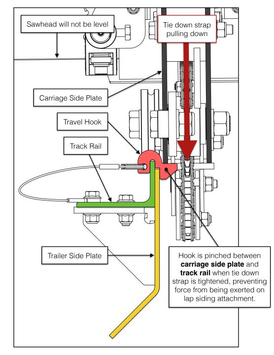
Note that the carriage will <u>not</u> sit level when locked-down for transport. This is normal.
