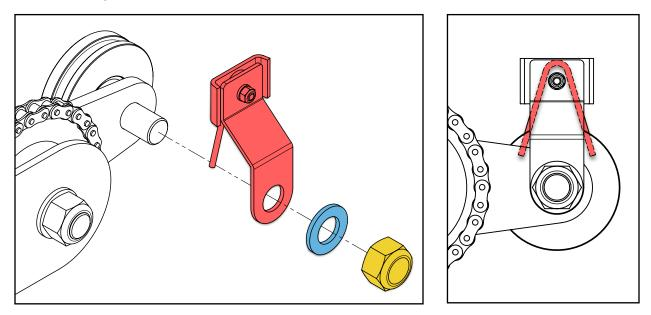
On the rear carriage wheel, turn the wheel sweeper assembly so that it is angled approximately 20-30° from the rear carriage post. Ensure it is oriented as shown to avoid the rear idler. Fully tighten the hardware.
