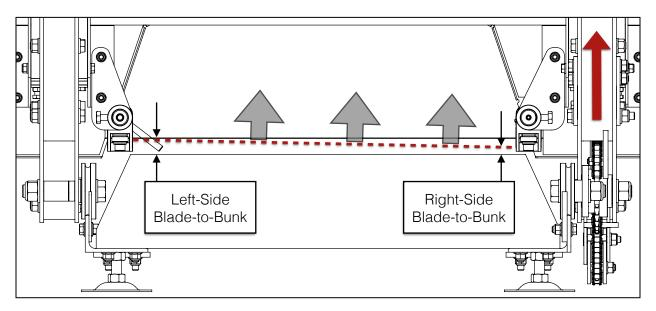
Turn the tuning block bolt clockwise to raise the sawhead until it is level. Once level, tighten the jam nut.
