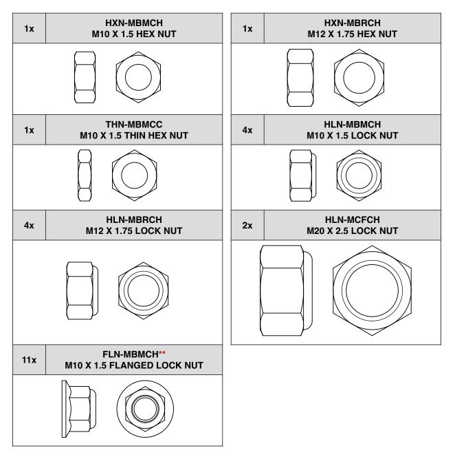
\*\* Total M10 X 1.5 Flanged Lock Nut quantity 9x on HM122 Lap Siding Attachment
