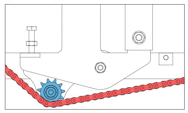
Like the rear carriage wheel, the groove in the front carriage wheel must also be seated down on the track rail as far as it will go. If the arm is rotated even slightly downward, remove the chain from the arm sprocket, rotate the arm until it is level or pointing just slightly upward, and then reset the chain.
