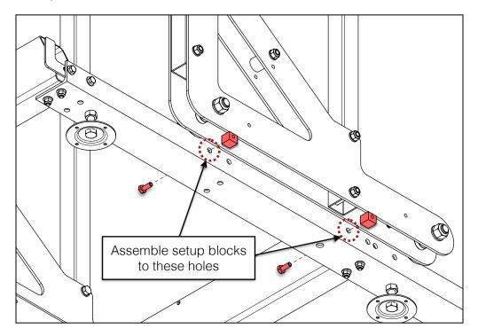
With the setup blocks in place, the inner carriage plate will support the weight of the sawmill carriage once the carriage wheels are removed. Note: the setup blocks sit approximately  $\frac{1}{8}$  in [3 mm] lower than the inner carriage plate prior to wheel removal—this is normal.
