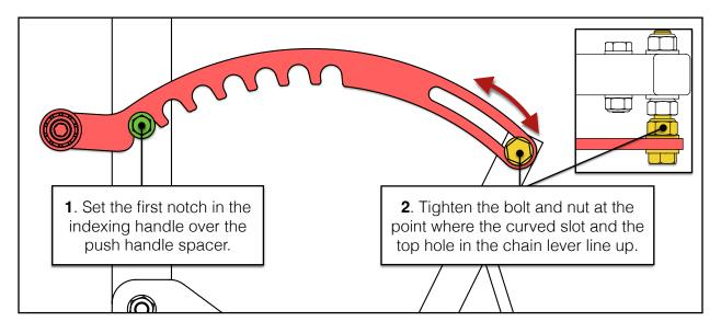
Adjust the middle and end nuts on the indexing handle to better position the handle over the push handle spacer. Fully tighten the hardware once positioned correctly.
