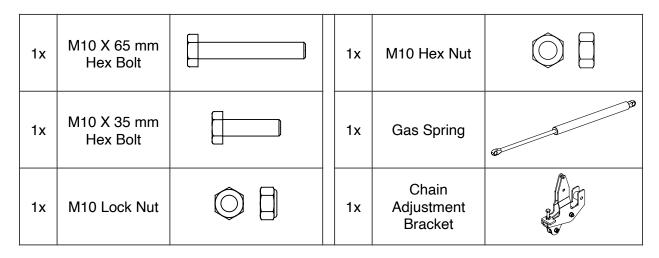
Assemble the gas spring to the chain adjustment bracket using one (1) M10 X 35 hex bolt and one (1) M10 lock nut. Take care not to over-tighten the bolt to ensure the gas spring pivots with ease.
